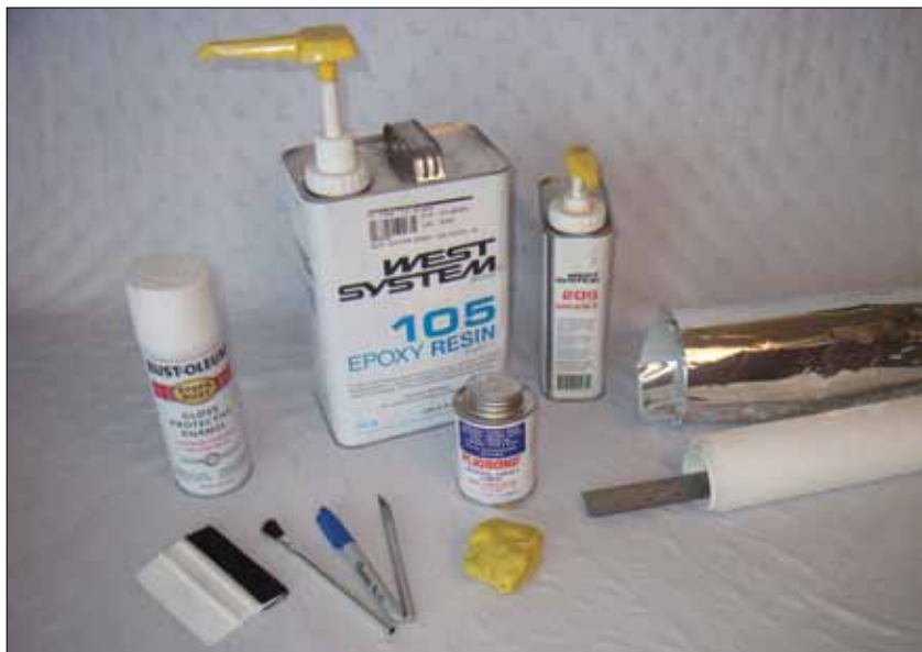
Here's what you'll need (clockwise): Laminating epoxy, adhesive-backed foil, Fiberfrax and a straightedge, a half pint of Plasti-Bond adhesive, modeling clay, a sharp X-Acto knife for trimming the foil, a Sharpie for template layout, an acid brush to seal the edges of the foil with epoxy, a window-tint applicator, and paint.
