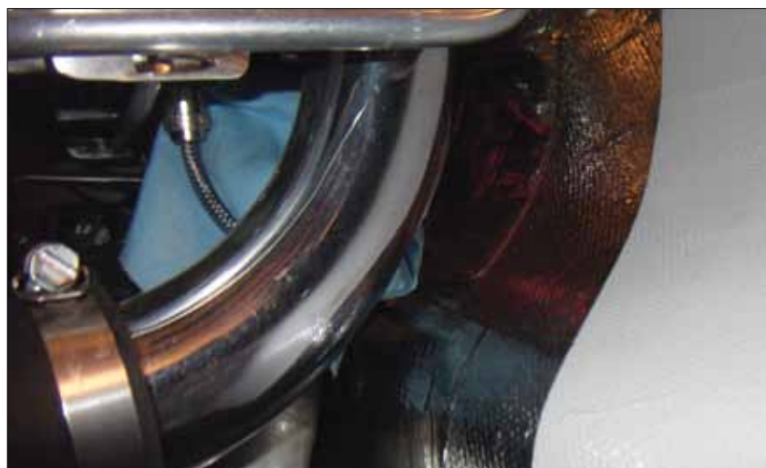
Close-up of Fiberfrax/foil barrier adjacent to an exhaust pipe. (Pipe hidden behind intake runner.) Epoxy to seal the edge has not yet been applied in this picture.
