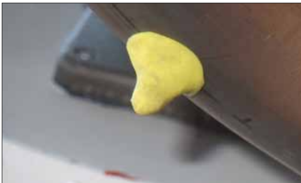
Clay cone stuck to the exhaust pipe to check for clearance.
