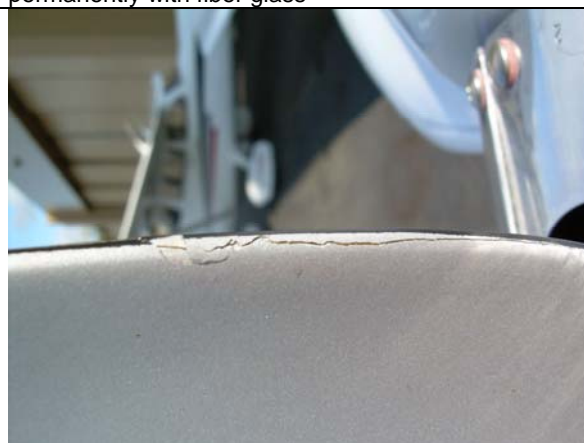
Damage caused by Cowling, seal and fill up with epoxy
