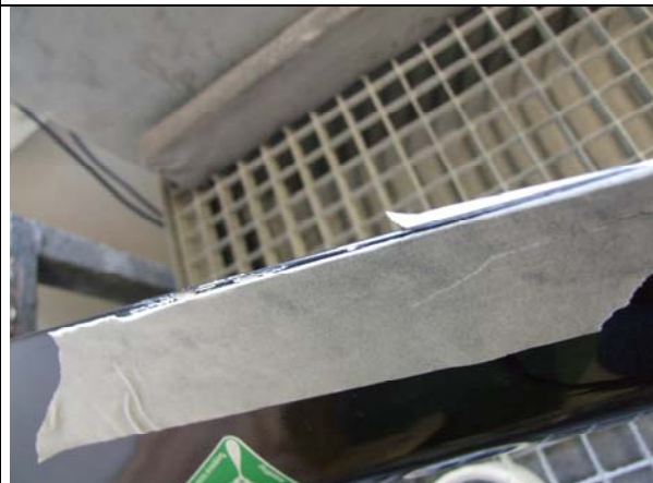
If the fiberglass shell on the trailing edge is delaminated the shell may be rebonded. Let pour 5 minute Epoxy into the trailing edge crack.
