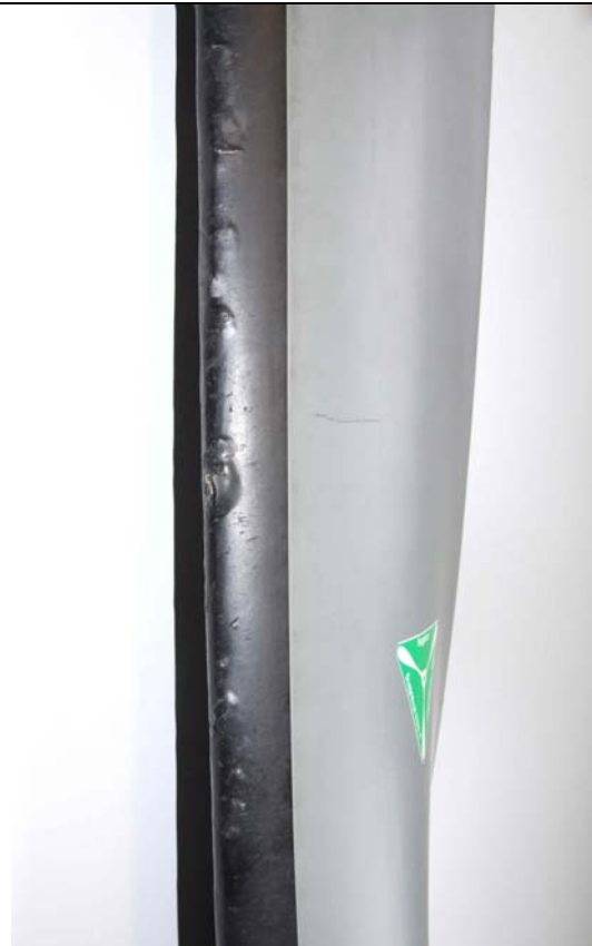
Typical Damage: Punched through PU-Strip
