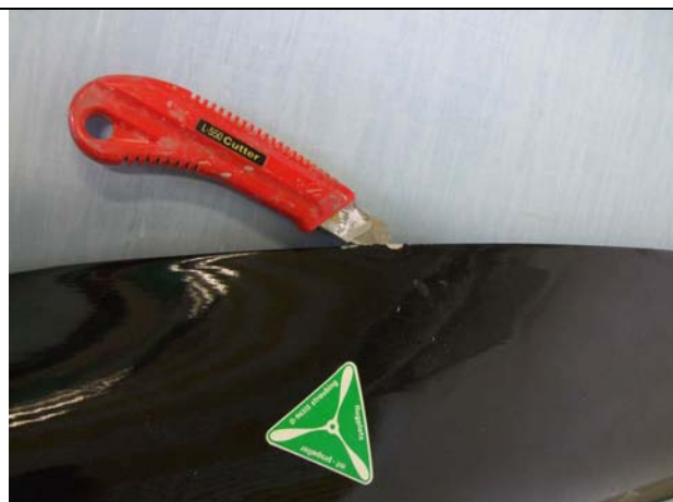
Delaminated composite shell on the trailing edge
