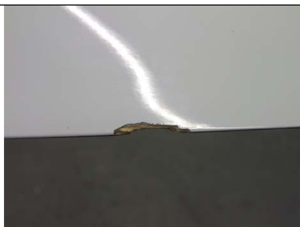
Tow bar damage, seal with Epoxy or repair permanently with fiber glass
