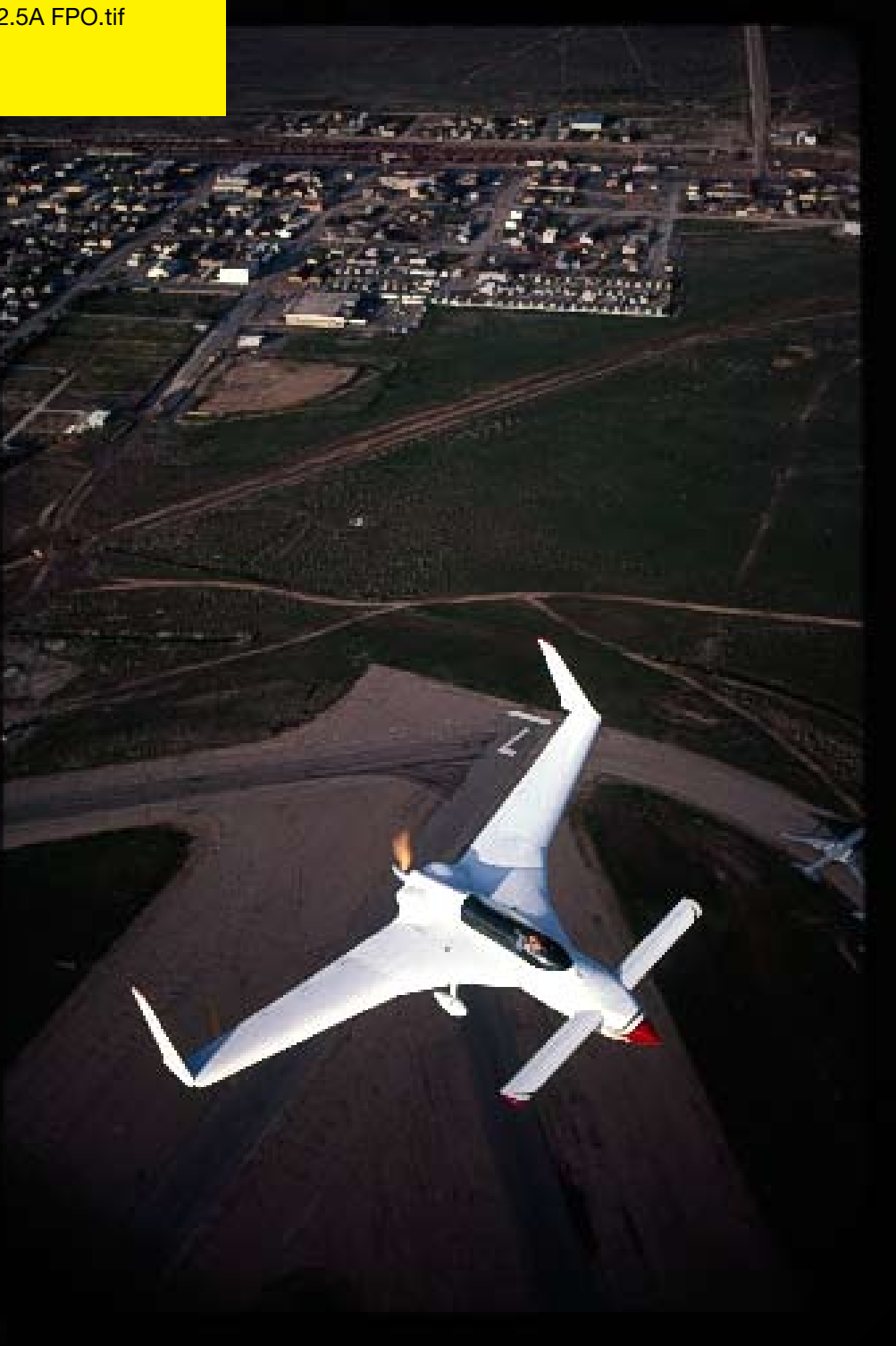
The last of the “EZ” trilogy, the Long-EZ had a cruising speed of 184 miles per hour, which was 9 miles per hour slower than that of the cruising speed of the VariEze homebuilt, but the Long-EZ more than made up for it by having a range of 1,970 miles, which was nearly double the range of the VariEze homebuilt. Courtesy of Burt Rutan
