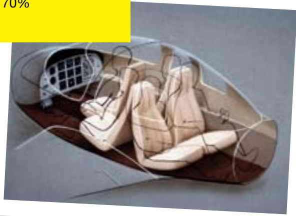
Even the seating of Catbird emphasized efficiency. The pilot and passengers were packed to minimize the required cabin space by considering the shape of people sitting down. So the pilot sat centered in front, giving the front row passengers leg room to the sides, and the back row passengers faced the tail with their legs in the narrowing part of fuselage. Courtesy of Burt Rutan
