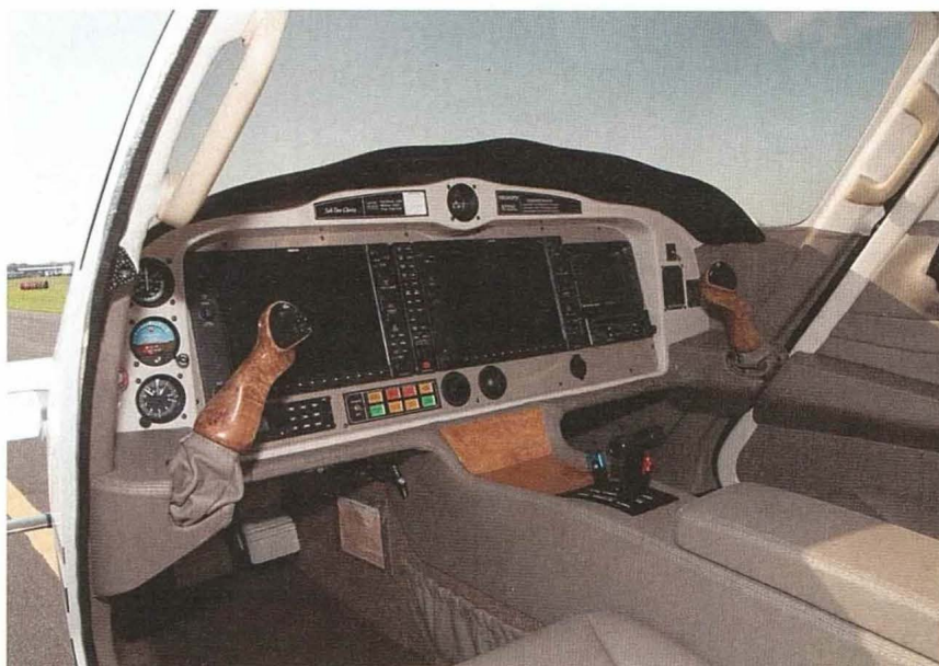
Top: The leather interior and Garmin G900X instrumentation makes for a comfortable, state-of-the-art cabin. Bottom: The Velocity has some of the slickest frontal aerodynamics of any aircraft, courtesy of its pusher configuration.
