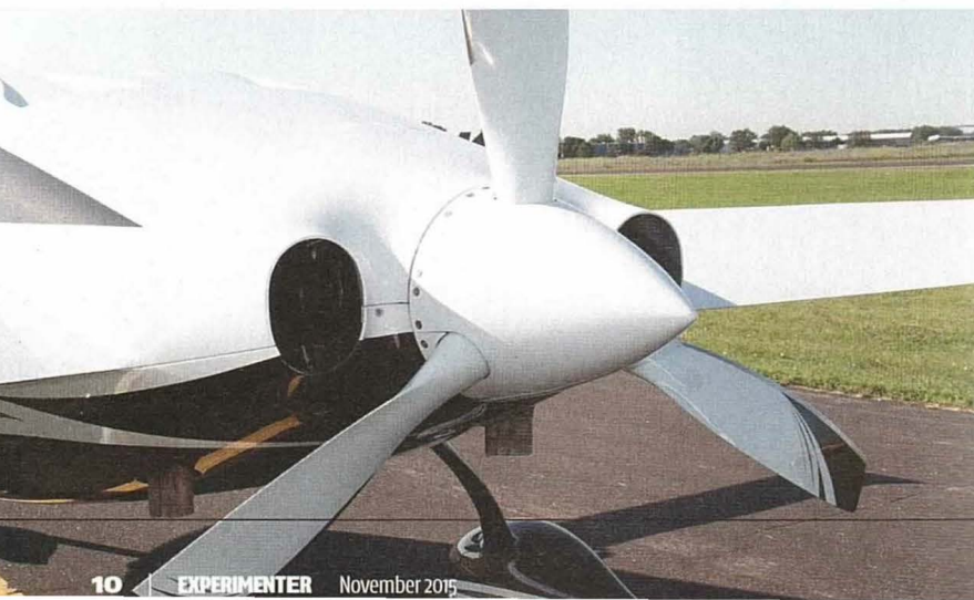
Bottom: The 70-inch AeroComposite constant-speed prop is driven by a 310-hp Continental IO-550N.
