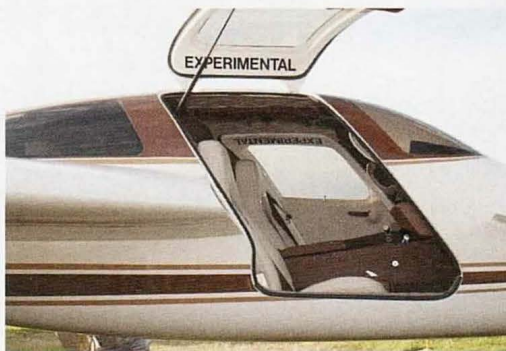
The XL cockpit/door dimensions, which are larger than many “normal” twins, were retained on the V-Twin.
