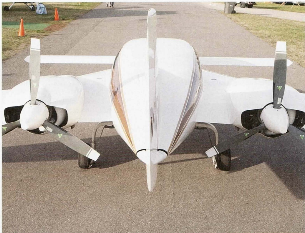
The engines are mounted closer than normal to centerline, which reduces asymmetric thrust with a dead engine.
