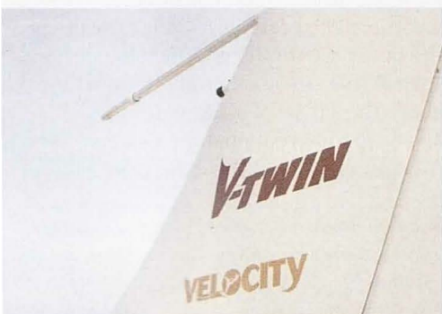
Winglets were replaced by a large central fin and rudder to give sufficient control with one engine out and the other at full power.
