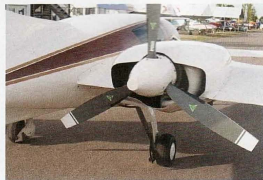
The 160-hp, fuel-injected Lycomings are burning 6 gallons each at 175 ktas, or 8 gallons at 185 ktas.
