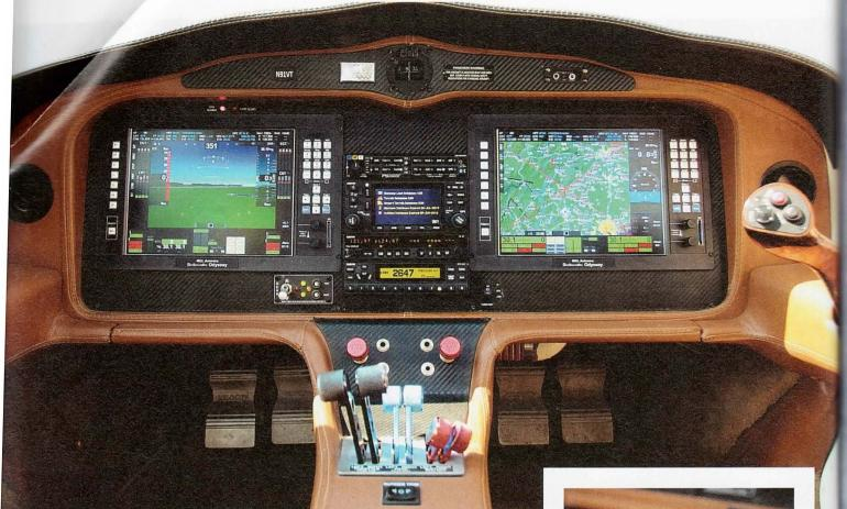
**AN MGL AVIONICS** suite is the centerpiece of the all-glass panel in the Twin Velocity prototype (above), although builders may choose between a wide variety of FAA-certified and Experimental avionics. The throttle, prop, and mixture controls are mounted in the center of the cockpit and the airplane can be flown from the left or right seat via sidestick controls (right). A door on the aft center console opens to reveal a bank of circuit breakers (below right).
