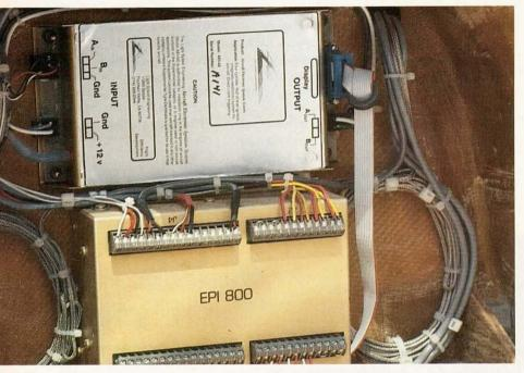
Engine sensors connect to this data-processing unit located behind the rear seat. A single ribbon cable runs to the panel where it attaches to the individual Vision Micrsystems display faces. neberg from having to maintain an inventory of thousands of dollars worth of expensive carbon-fiber components.
