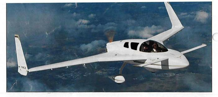
condition. Continued pull to full aft stick (20-25 lbs.) has little effect on airspeed which varies from 60 to 63 knots on the indicator during the pitch oscillation. With full aft stick held, the airplane's average pitch attitude varies a couple of degrees. At 60 knots the nose wanders down until the airspeed increases to 63 knots, then the nose wanders back up, and the cycle repeats with the pitch bobble continuing throughout the slower average pitch attitude oscillation.
