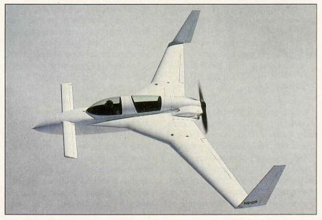
Wingspan is 26.6 feet of high-modulus carbon fiber that enables the Berkut to cut through turbulence with minimum loss of airspeed.
