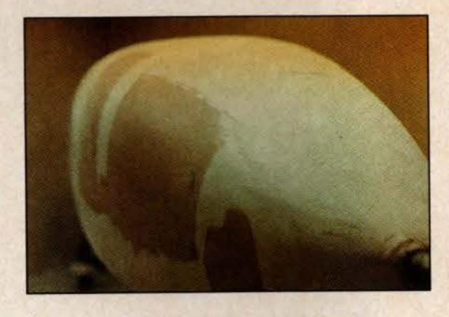
The shape of the Berkut was transferred from paper to reality via this fuselage plug. Still unfinished, it was used as the form for making the female molds.
