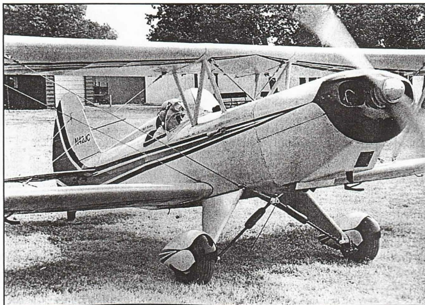
Don't blast your throttle to get the airplane rolling. Prop vortices will suck up dirt and pebbles even on paved surfaces. Use minimum power to get the airplane moving...then smoothly increase power to keep it rolling.
