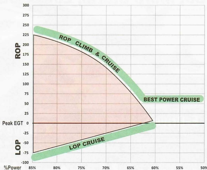
Figure 4—The three most useful outside-the-red-fin zones for climb and cruise.
