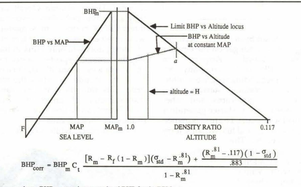
where:  $BHP_m = maximum$  sea level BHP for the RPM
