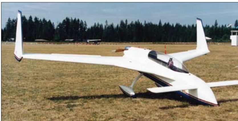
The Rutan Long-EZ was an outgrowth of builders' desires to use larger engines than the VariEze could tolerate.
