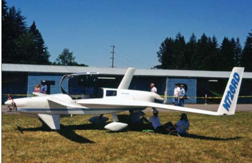
Rutan's ultimate Long-EZ evolution was the twin-engine Defiant. The original design used a forward rudder.
