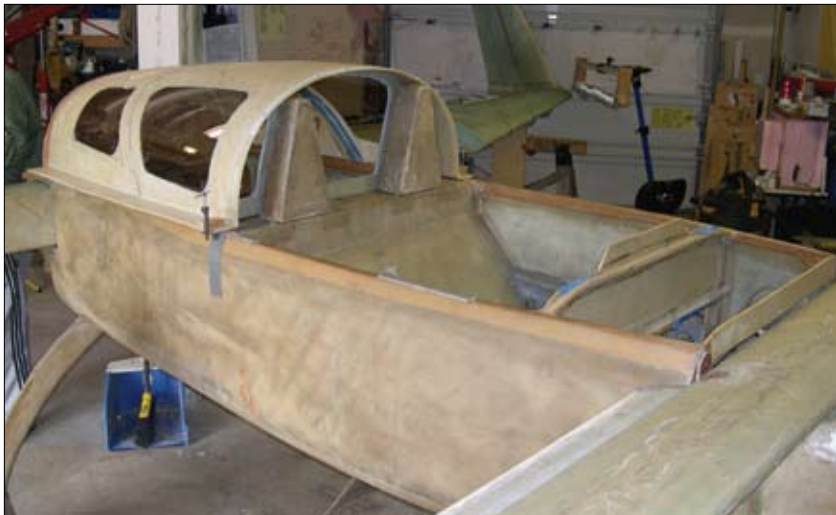
Rutan-inspired canard aircraft such as this Cozy usually include turnover structures built into the seats. This improves accident survivability.
