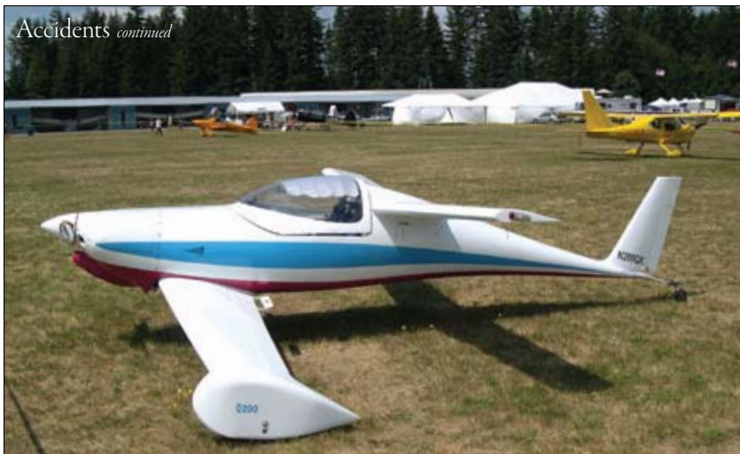
The Q200 was the two-seat version of the Quickie with a Continental O-200 engine. This version retains the original position of the main landing gear on the wingtips of the canard.
