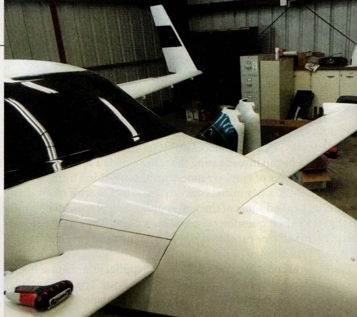
The access panel on the nose was the first section to be vinyl wrapped followed by the panel over the canard wing.
