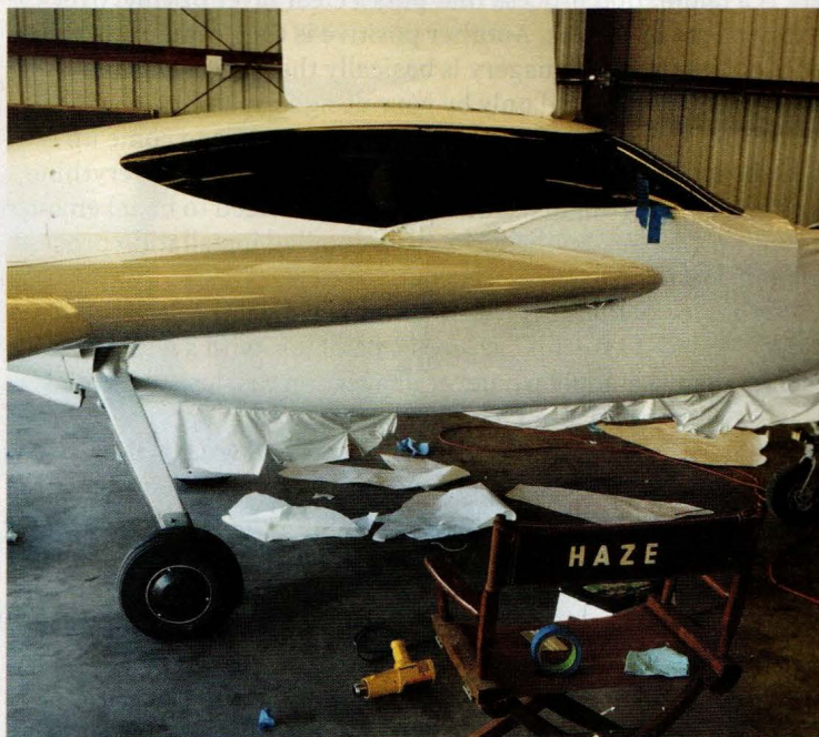
Above: The vinyl stretches to conform to the shape of whatever you're applying it to.
