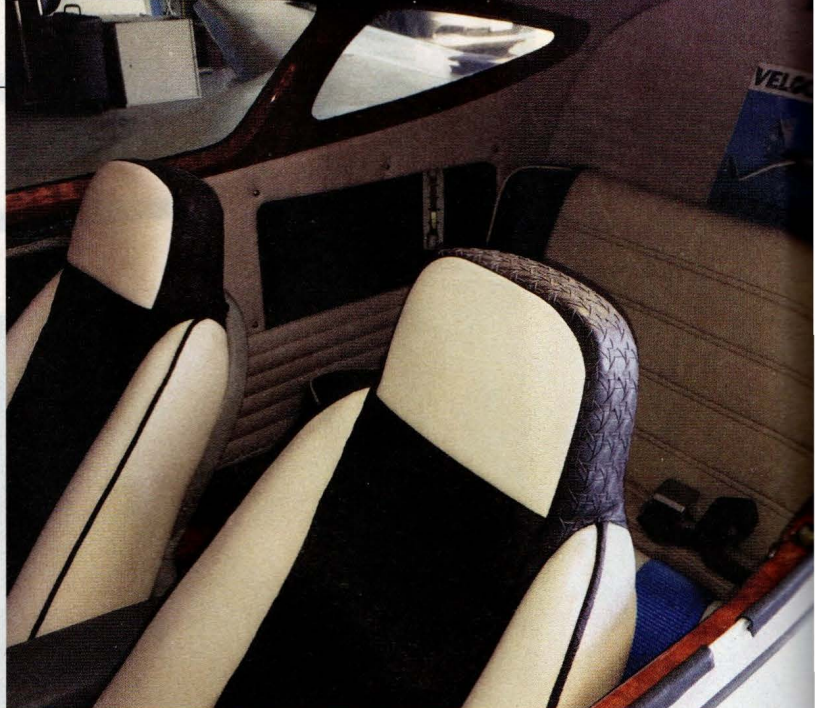
The seat upholstery is one of the few design elements I hired someone else to do. The burl wood window trim was created using vinyl wrap.
