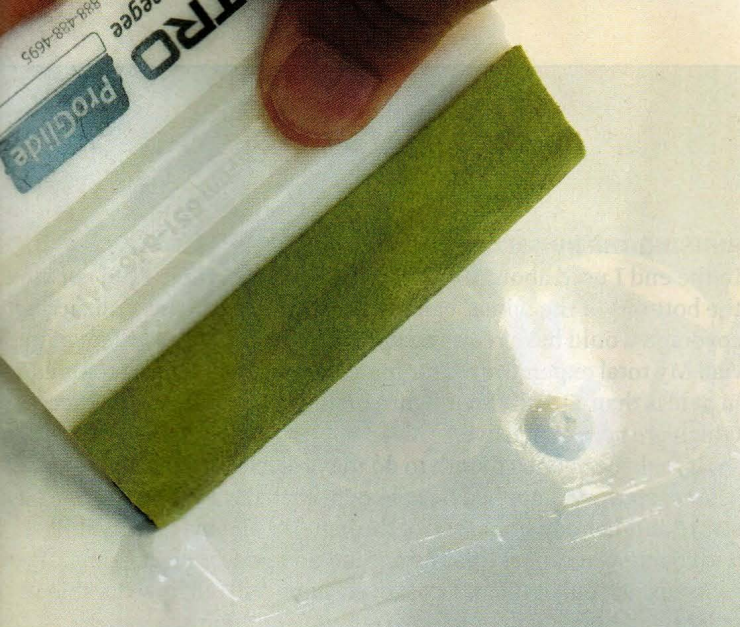
A felt-tipped squeegee was used to apply the vinyl to prevent scratches.
