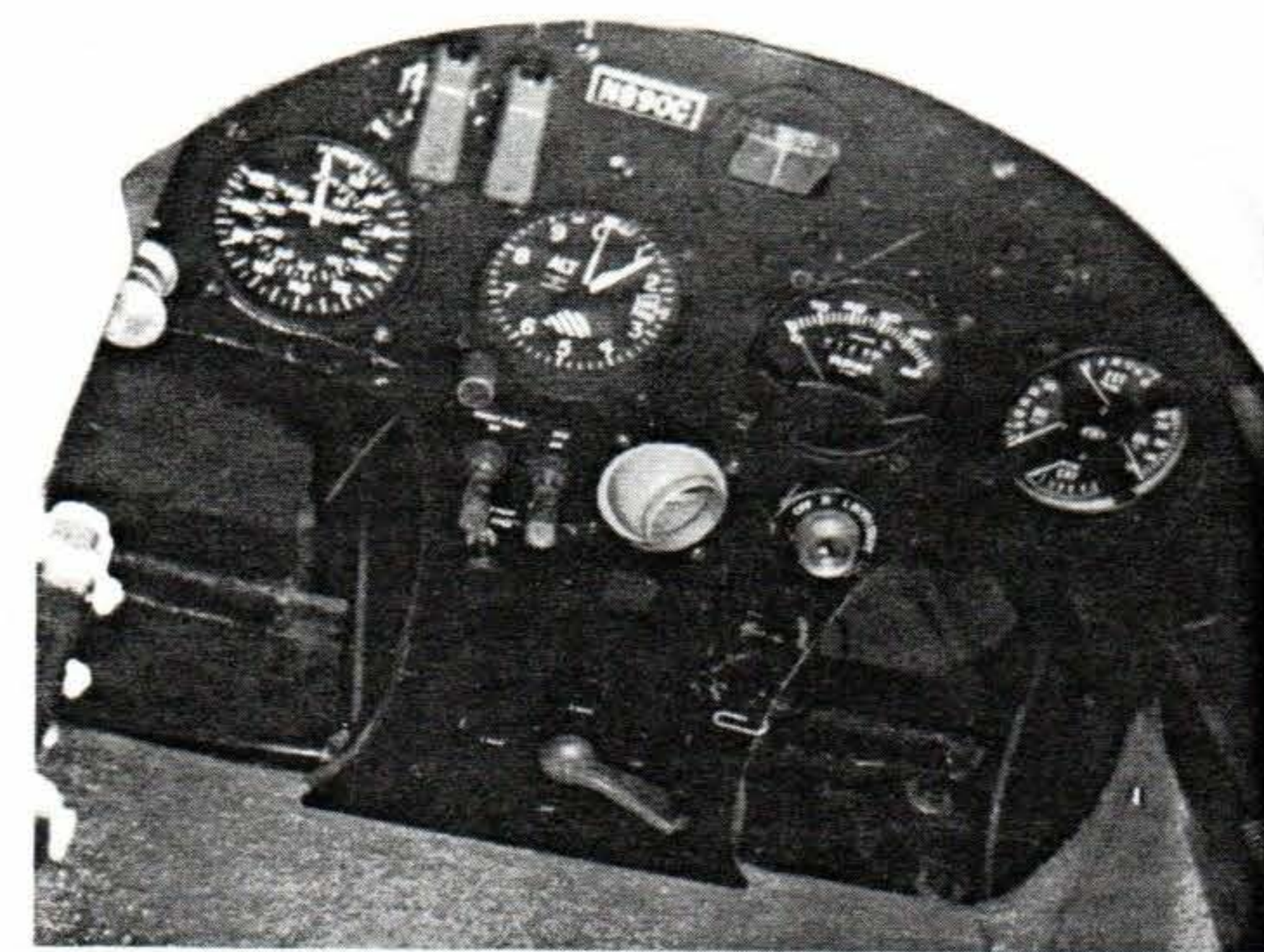
Fully adequate instrument panel for Arizona-Oshkosh and other X-country flights. Hand held NavCom radio (not shown) is normally connected to the external antenna.
