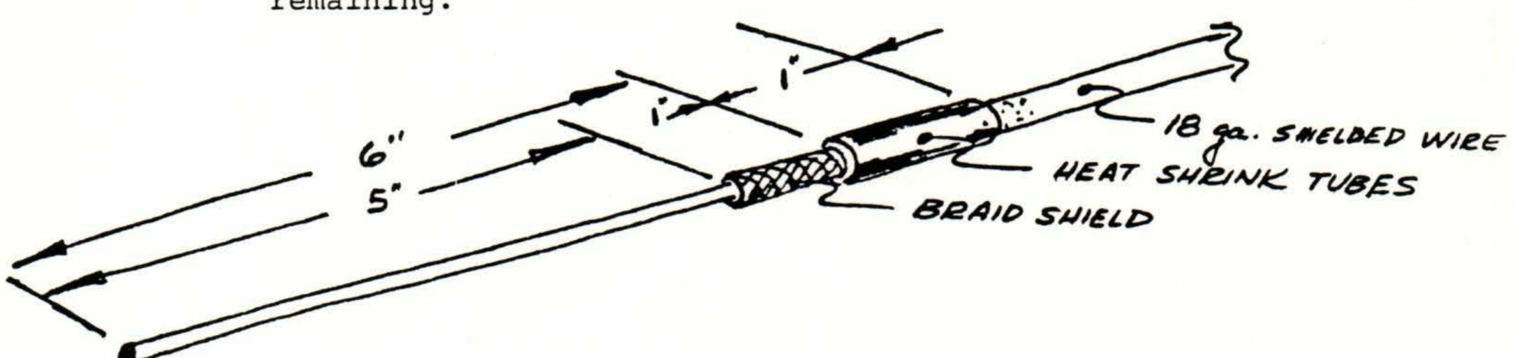
STEP 2 Cut 2 pieces of heat shrink tubing 1" long and shrink them both over the outer insulation as shown. Carefully unravel the remaining 1" of braid & fold it back over the heat shrink tubes. Cut a third piece of heat shrink tube 3/4" long and shrink it in place over the inner insulated conductor pushing the heat shrink tube as far under the braid as possible. You should now have this:
