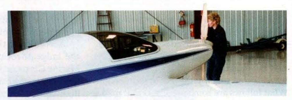
With small aircraft that use a propeller gear reduction drive, such as Rotax, pulling the aircraft around the hangar by the prop root may be permitted (check with the manufacturers of the prop and the engine). Traditional prop and hub arrangements should be moved using a tow bar.
