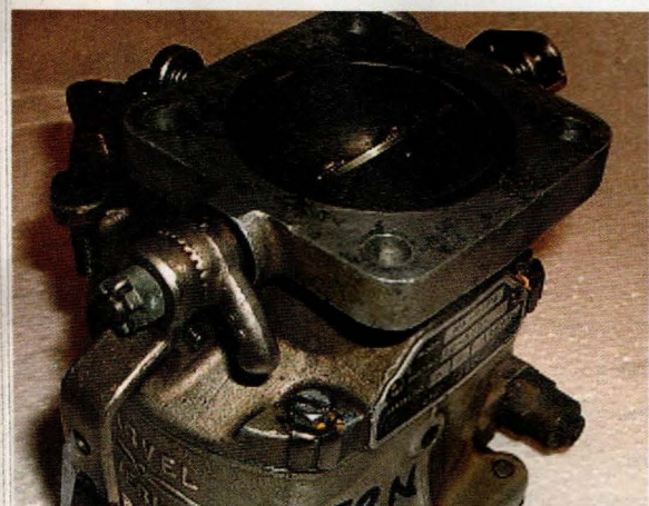
The O-320's carburetor was re-jetted to increase takeoff fuel flow from 12.5 to 13.5 gph.
