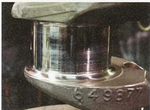
This Continental IO-360 spun a main bearing after cylinder work. Fortunately, the situation was caught at a routine oil change (where the filter was found to have thousands of flakes of bearing metal) literally an hour or two before the engine would have self-destructed in flight.
