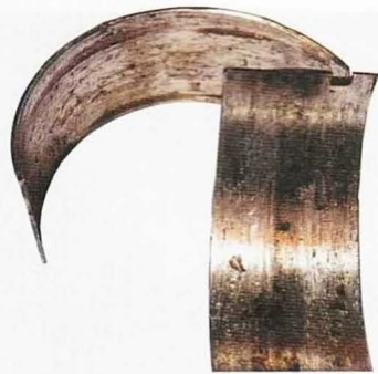
Figure 12—A badly contaminated bearing with large amounts of foreign material embedded in its babbitt overlay.
