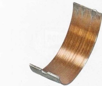
Figure 11—A severely worn bearing with the babbitt overlay almost completely gone.
