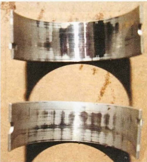
Figure 13—This bearing exhibits severe overload damage, probably due to detonation or preignition.
