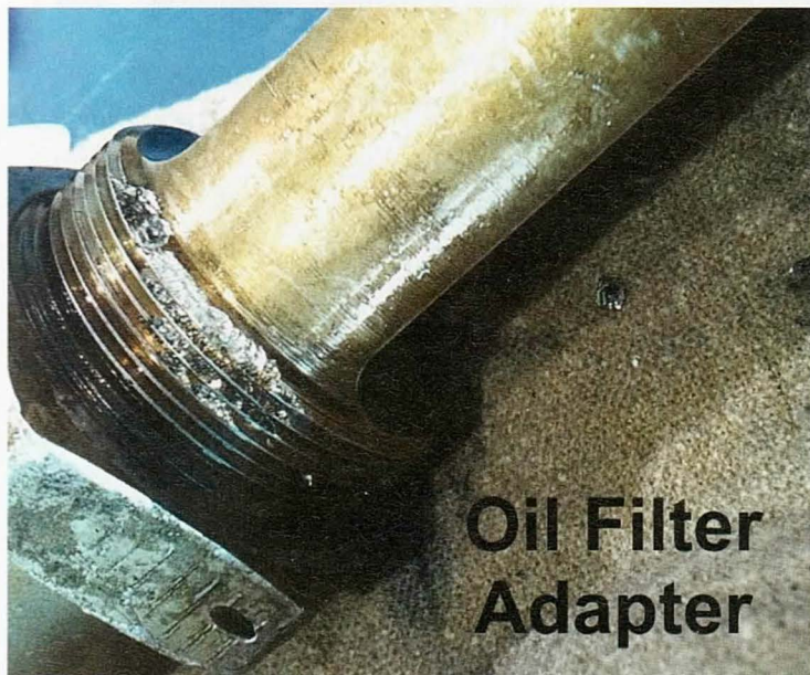
Source of the aluminum chunk found in the pressure relief valve: torn-up threads in the oil pump caused by a loose oil filter adapter. Mystery solved!
