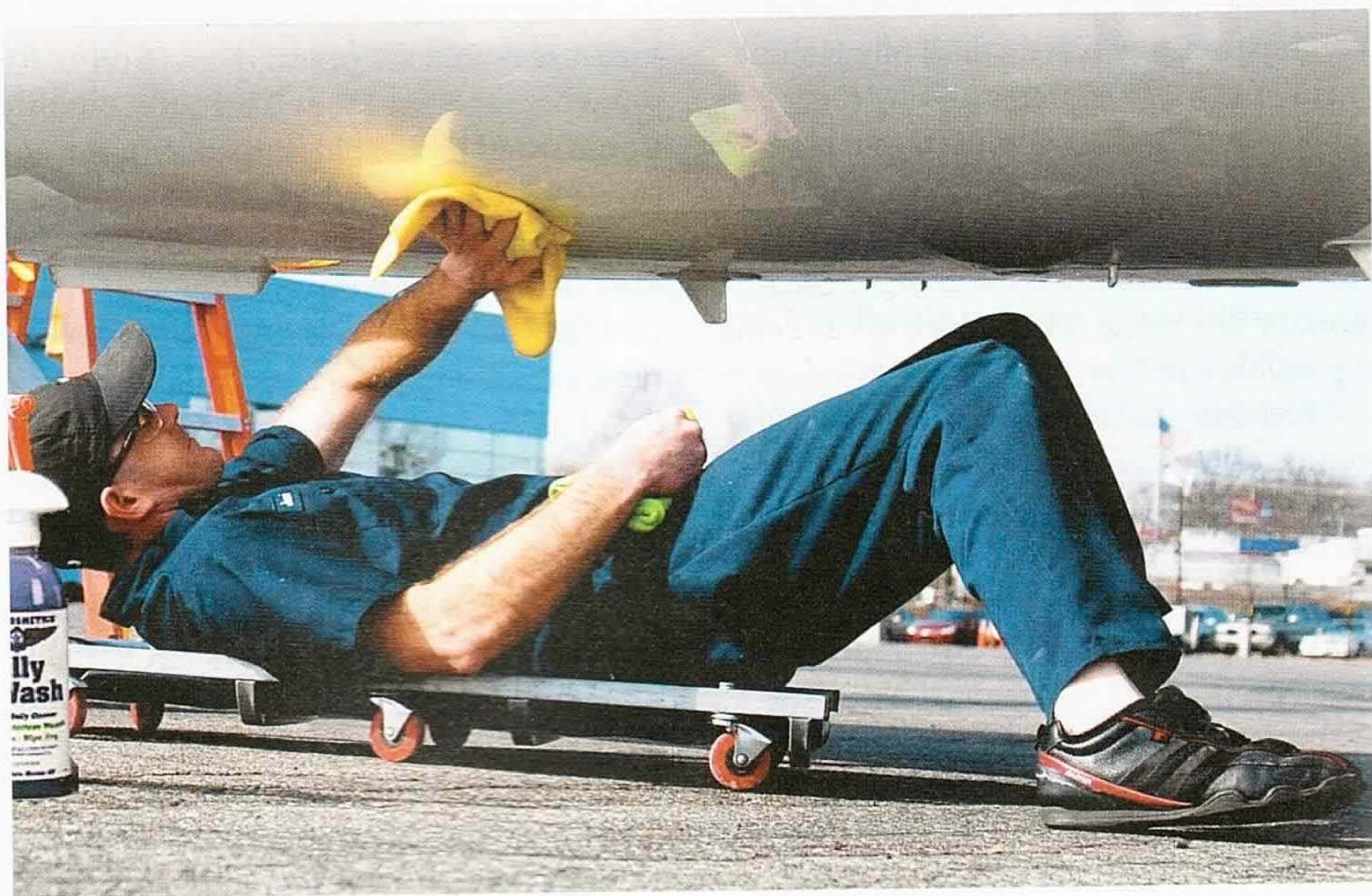
Excessive discharge of oil on the belly is often caused by excessive blow-by in one or more cylinders—but not always. Unless the oil is turning dark and opaque very quickly after each oil change, blow-by probably isn't the cause.
