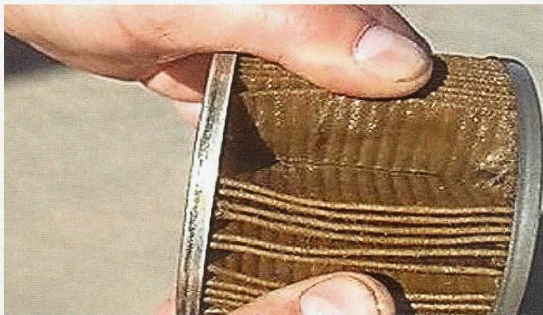
After a 30-minute ground run and a full-power high-speed taxi run, the oil filter was spotless.
