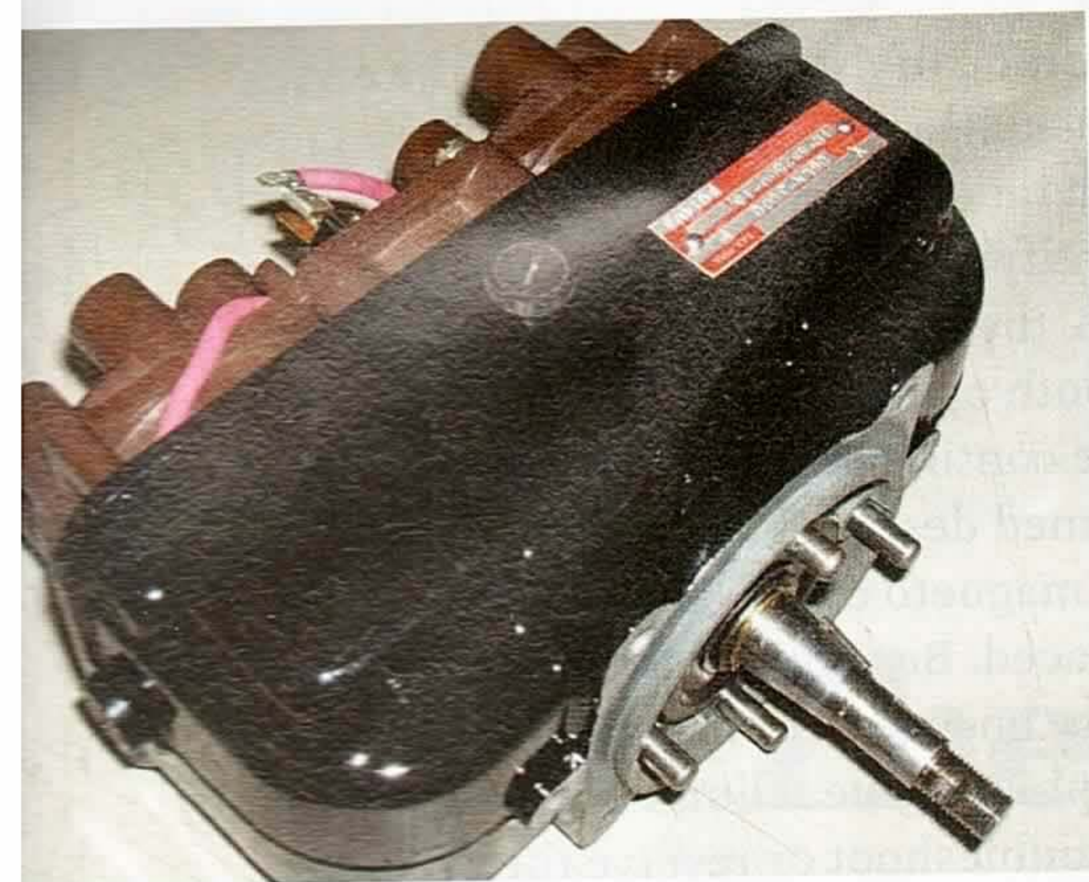
Figure 2—The Bendix D2000/D3000 dual mag is basically two independent magnetos packaged into a single unit.
