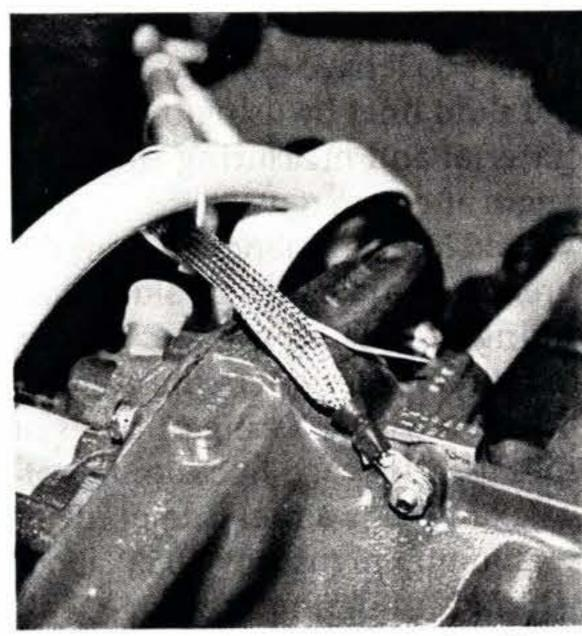
The engine grounding strap should electrically connect the engine with the firewall. Composite aircraft usually ground the engine to the battery.
