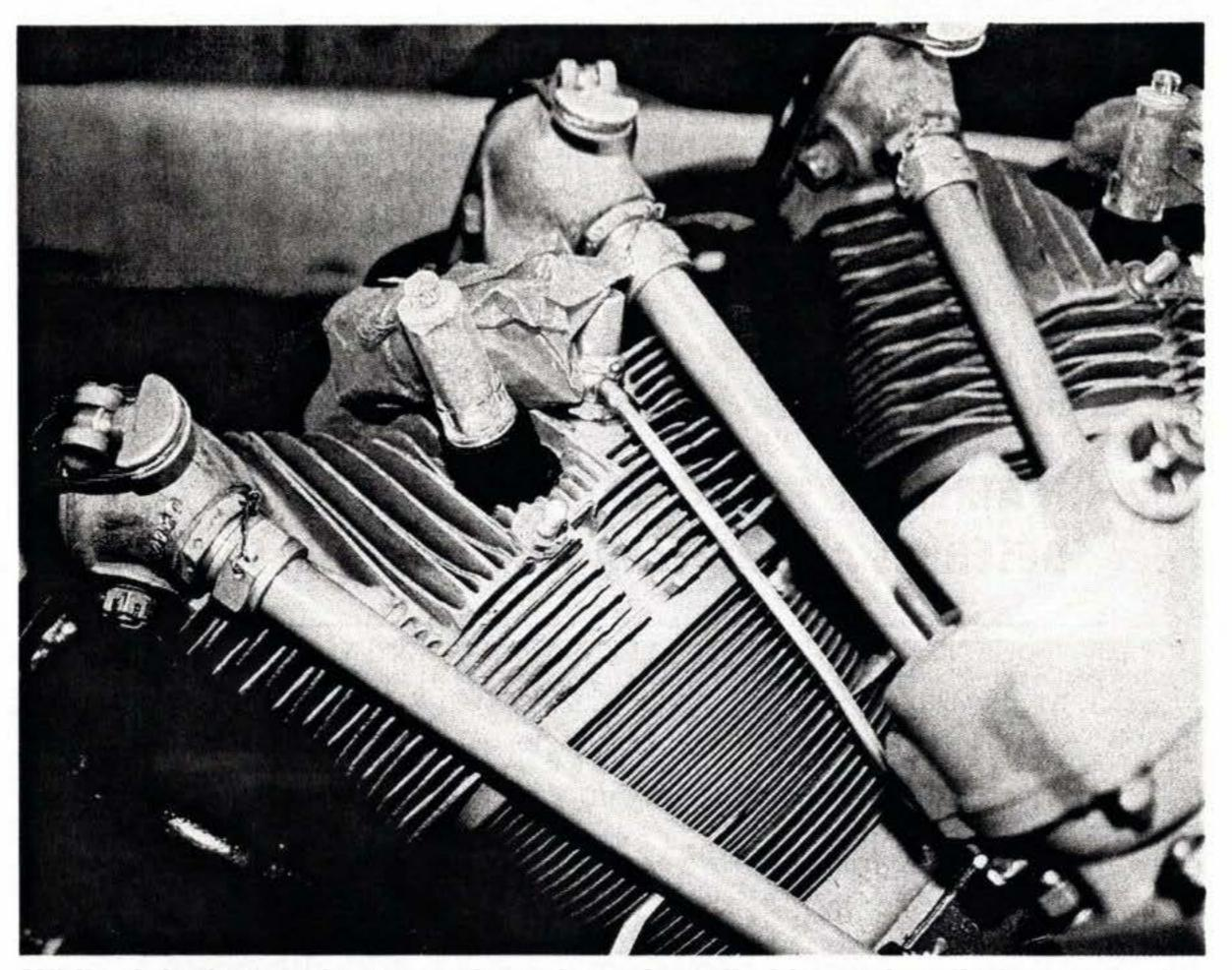
While dehydrator plugs may have been installed in each cylinder to ward off moisture, your engine might also be filled with preservation fluid. Remove the plugs from the lower cylinders and drain the fluid *before* turning the crankshaft.
