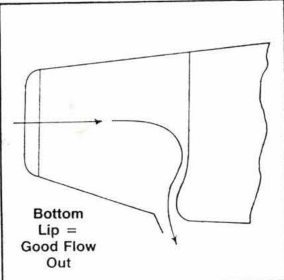
At high speed the air has to turn a corner getting into the cowl and if too much air gets in, it must go out again around the cowl. If that edge is sharp, the drag rise will be high.
