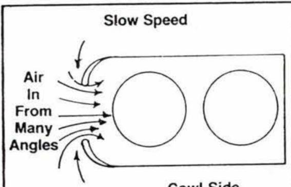
In the Sonerai newsletter, there is information on how small vortexes caused stagnation and hot spots on cylinders due to poor baffling.
