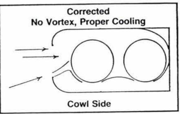
EAA Director Harry Zeisloft designed a bottom lip for good flow outlet that had considerable performance effect on both cooling and cruise speed to eliminate the sharp lip at the bottom of the cowl. Slow speed air comes in from all around the cowl and it needs the curved inlet lip there as much as any.
