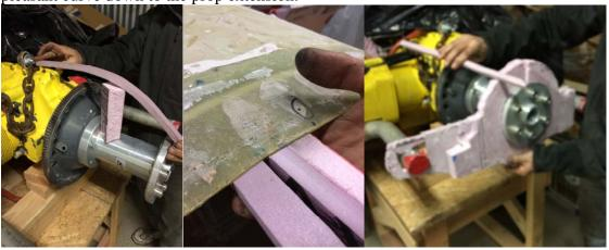
5) You may not need this step but my 540 cowl is a bit longer. I made a piece of foam for each side the shape of my wing root to trailing edge then made it about 6 inches longer. On this photo you can see it attached to the firewall at the same level and width of the spar. I made sure the "point" was level with the trailing edge then supported it with more pieces of foam and the glue gun. Notice in this pic I have the NACA blocked with a piece of foam as the attach point for the center strips.
