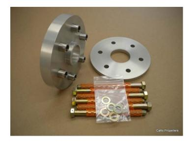
The 1" spacer kit is a very simple installation and easily snaps on the face of the starter ring gear of the engine. The new face on the 1" spacer kit has the longer  $\frac{3}{4}$ " lugs and is 7" in diameter to match the 7" diameter face of the propeller. The kit also includes either a  $\frac{3}{8}$ " or  $\frac{1}{2}$ " thick crush plate and new longer propeller bolts.
