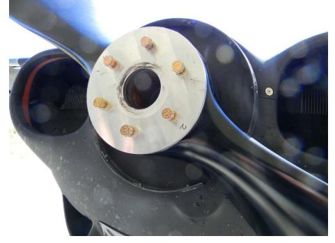
2.3.5 Place the spinner front bulkhead (if needed) and crush plate on the opposite hub face and insert the bolts through the assembly.
