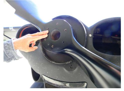
2.3.4 Ensure you have minimum 1/2" inch of lug engagement into the propeller hub face. These lugs are either 5/8" or 3/4" inch in diameter and protrude from your engine flange or propeller extension or spacer.
