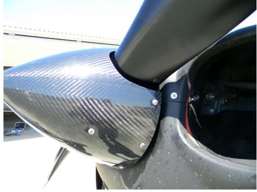
2.3.11 Check bolt torque after first 2 to 3 hours of operation and then again at 10 to 15 hours. After that, it is mandatory to recheck the bolt torque every 50 hours or 6 months, whichever comes first.
