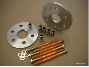
The ETP Kit consists of a set of new longer  $\frac{3}{4}$ " diameter engine lugs. A 7" diameter x  $\frac{1}{4}$ " thick aluminum plate is placed over the lugs before the propeller is bolted on. This now gives you the 7" diameter mounting face you need along with proper lug engagement into the propeller. On the outer face of the propeller is the  $\frac{3}{8}$ " or  $\frac{1}{2}$ " thick x 7" diameter crush plate. Also, included in the kit is your new propeller bolts.
