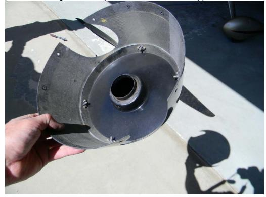
2.3.6 Using the standard ratchet, tighten all the bolts using a star pattern until the propeller and spinner assembly are snug. Ensure that the propeller bolts have adequate overall length (minimum 3 threads out the back). Verify that the propeller bolt threads do not "bottom out" onto the threaded engine or extension lugs. Verify thread length does not interfere with the engine case or impede movement of the propeller with surrounding components.
