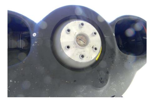
2.3.2 If a spinner is used, place the spinner rear bulkhead onto the engine flange. Orient the bulkhead so that the propeller blades will be aligned at the 10 o'clock and 4 o'clock positions as depicted on the propeller orientation mark on the crankshaft plug.
