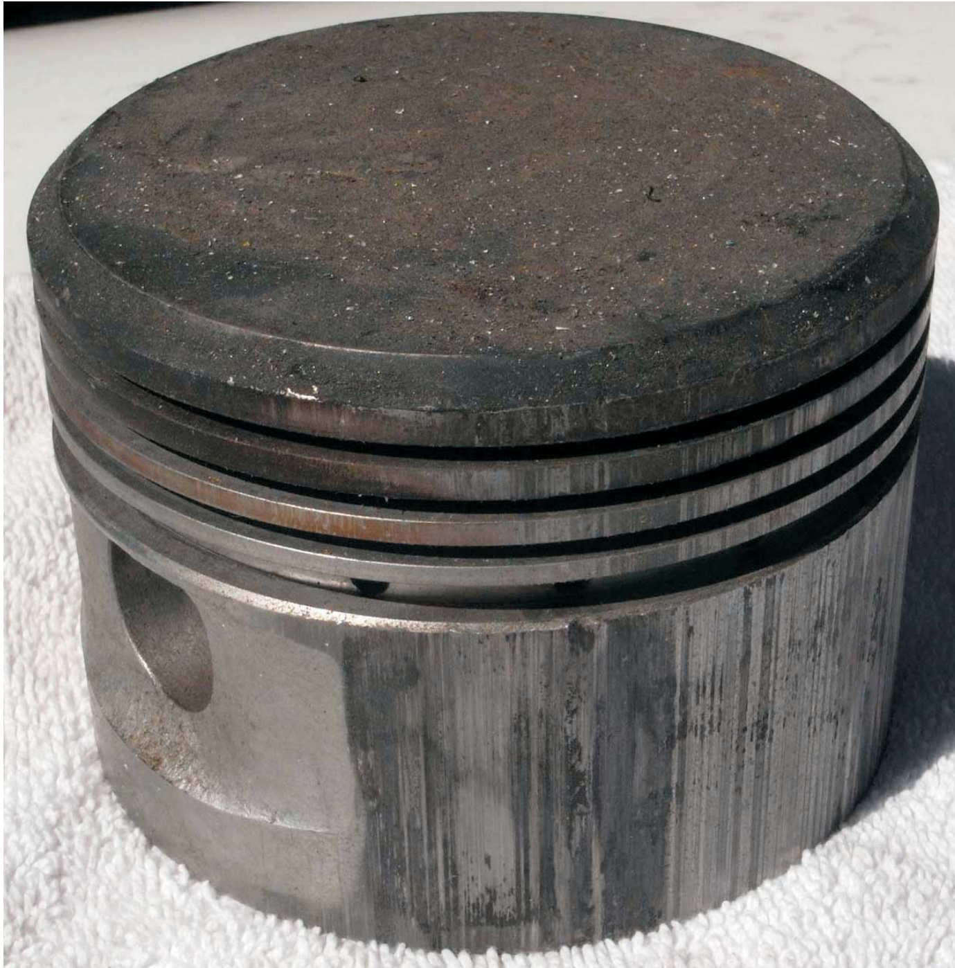
Aero Shell Oil temp peaked at 250°C. Piston Seized.
