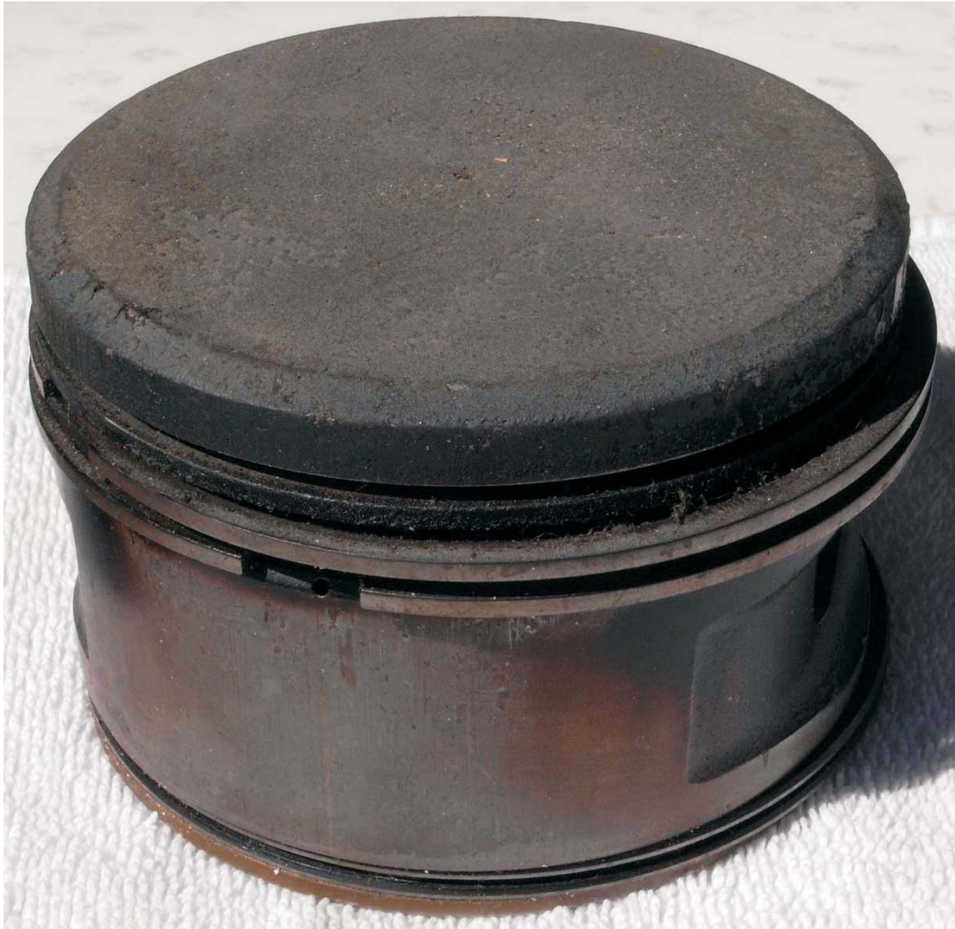
Aero Shell Oil temp peaked at 240°C. Piston TT 100 hrs.
