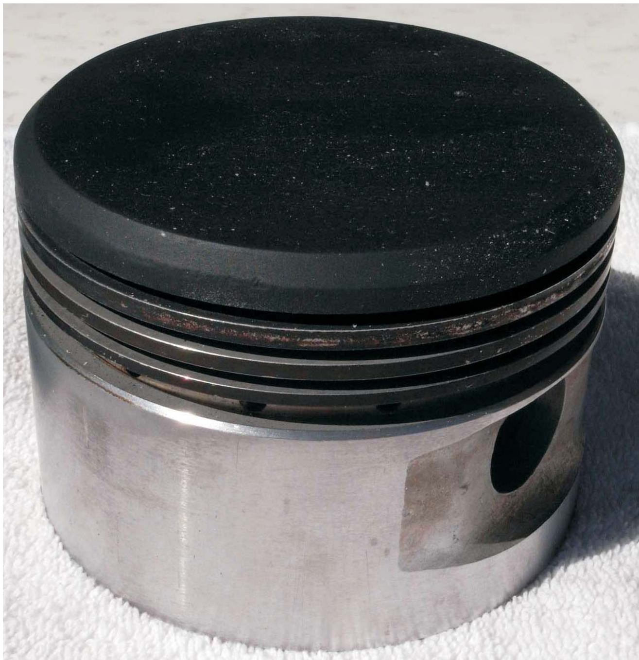
MOBIL1 Oil temp in excess of 260°C. CHT 540°C Piston TT 200 hrs.
