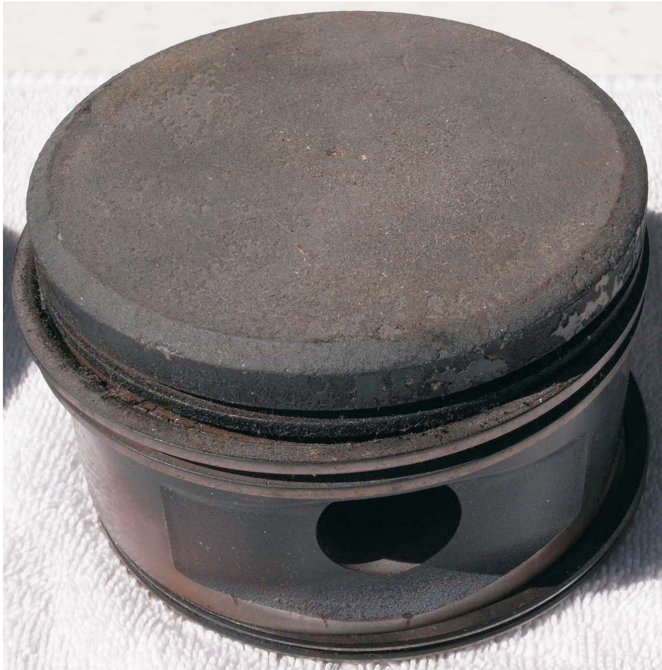
Aero Shell Oil temp peaked at 240°C. Piston TT 100 hrs.
