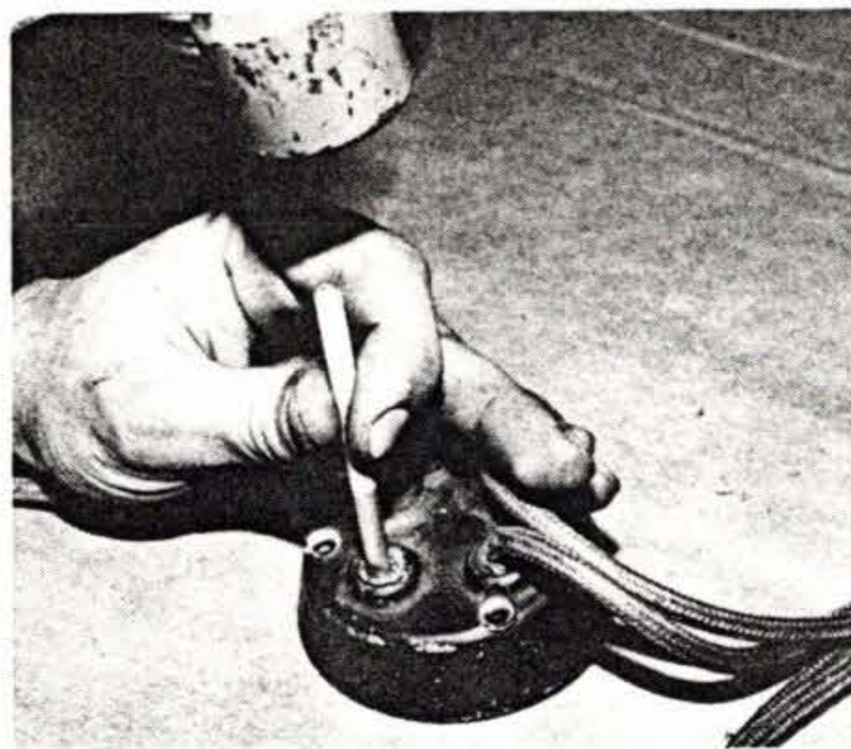
Above: The T-115 spring assembly tool can be used to punch the old drive ferrule out of the harness cap.
