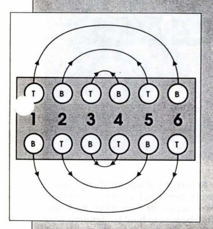
Owners of six-cylinder engines should rotate plugs as shown here, but first they should be arranged in the top and bottom orientation depicted. (Note the Ts & Bs in the little circles.) This scheme assures polarity alternation.
