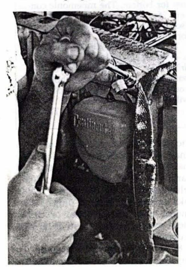
Application of Champion 2612 thread lube should begin a minimum of one full thread away from the firing end. Some people use Dow DC-4 or DC-10. Engine oil will tend to turn to coke, cementing the plug in place; if you use engine oil, be sure it's synthetic. Your torque wrench (below) can be 3/8in. or 1/2-in. square drive. The important thing is that it is accurate in the 25-35 ft-lb range.
