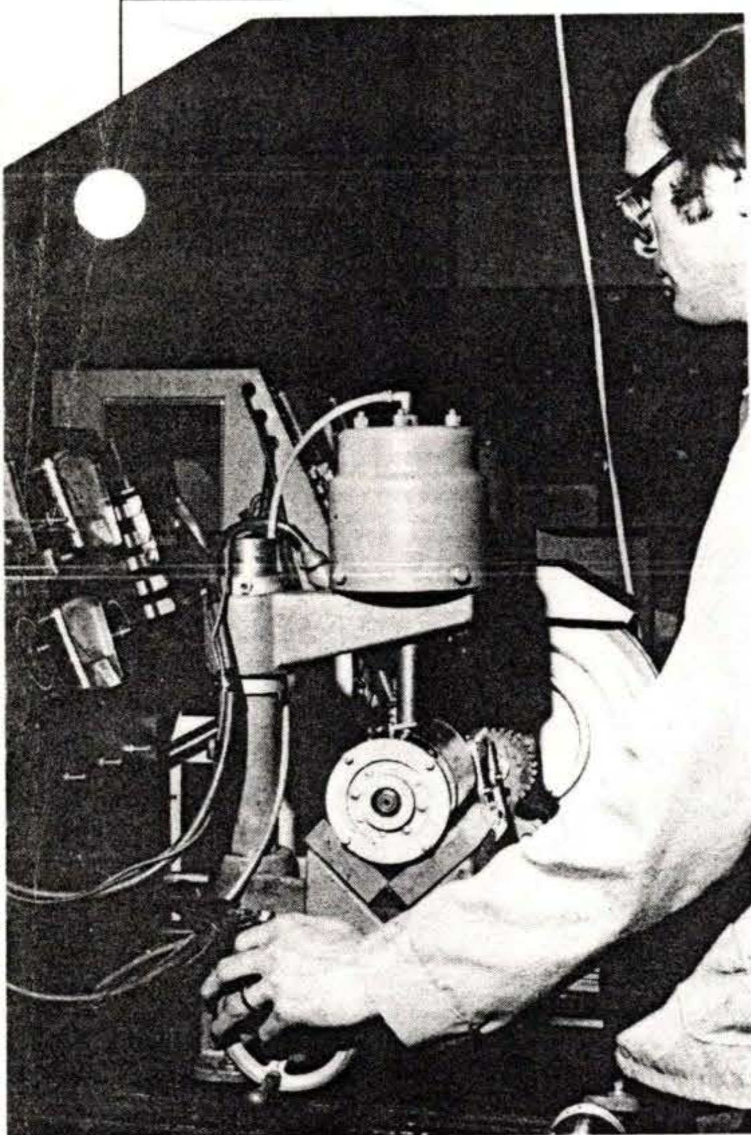
Proper testing of a starter motor includes a bench check of stall torque, stall amperage, and no-load rpm.
