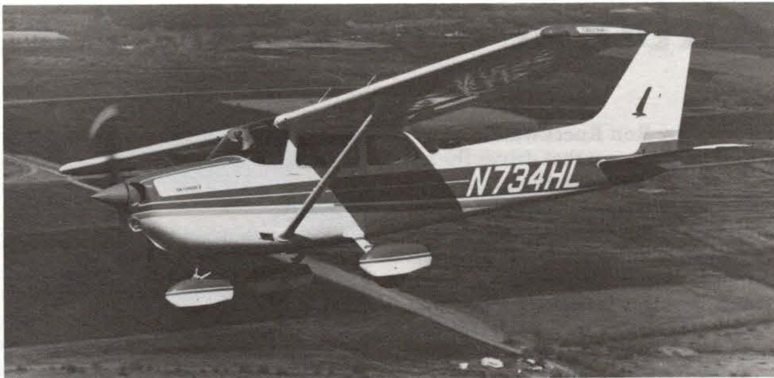
The Skyhawk's 150-hp Lycoming O-320-E2D can be converted to 160 horsepower relatively economically through RAM's piston-swap STC.
