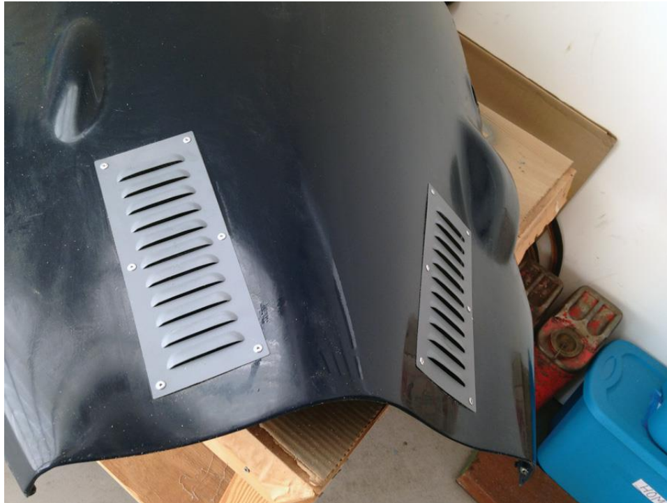
Small louvers on the bottom rear of the cowl helped draw air out.
