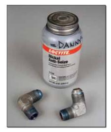
If aluminum fittings are the only option, anti-seize lubrication is a must. Even with this thread lube, the chances of galling the threads in the cooler are a near certainty. There's slim hope of repairing such damage with a thread insert because its installation generates too many metal chips.
