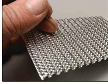
Tiny passages in the turbulator plate form a mesh the oil must pass through, which is too tight for .032-inch safety wire to penetrate, save at an extreme angle. It's these many small orifices that accumulate gunk after years of service and aren't going to be cleaned by a few hours in a solvent tank.
