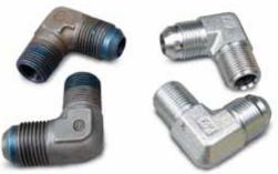
Pacific Oil Cooler Service notes their number-one issue with installations is thread-galling aluminum AN fittings (left). They are adamant all fittings must be steel (right) because steel fittings never gall the cooler's aluminum threads, even after many decades. They install steel fittings dry, or with red Loctite. If steel fittings seem too tight to remove safely, Pacific says a little heat from a torch does the trick.
