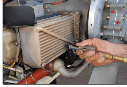
Corrosion starts on the outside of oil coolers when moisture-trapping dirt becomes lodged in the cooling fins. Pacific Oil Cooler Service says the cooler core should be cleaned with soapy water and blown dry at annual time. Work gently around the fragile fins, but otherwise this is a simple job an owner can do. Corrosion is what caused our cooler to spring a leak in flight, something you want to avoid.
