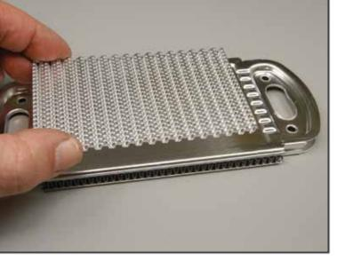
A turbulator plate is placed into a recess in one section of a drawncup cooler. Oil flows along the major axis of the turbulator plate, squeezing through the numerous holes in it, thus increasing the oil's contact with the cooler's surface area. Cooling air flows through the sine-wave-shaped fins in the drawn-cup section.
