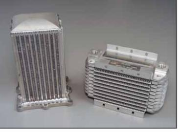
Continental oil coolers, left, are engine-mounted and of bar-andplate construction. Lycoming engines use remote-mounted oil coolers, typically, but not necessarily, of drawn-cup build, as seen on the right. Remotely mounted coolers require more savvy from the aircraft builder to properly integrate into the airframe, but allow Experimenters more freedom in under-cowl packaging.
