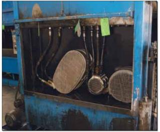
These giant coolers are old-school tube-type units, likely off a DC-3. They're being internally washed in a flushing bench at Pacific Oil Cooler Service. Pacific runs coolers through four different flushing stations until nothing larger than 10 microns comes out.
