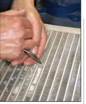
Straightening fins is a tedious, timeintensive job, but necessary for maximum cooler performance. It's also something you can do as there is no special skill or tools involved; simply guide the bent fin straight with a thin metal or wooden tool.
