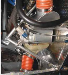
Swapping the bar-and-plate cooler resulted in almost no visual change, but the barand-plate's minimally-taller cooler height (firewall to hose fitting dimension) meant enlarging holes in the top and bottom air ducts, re-rigging the mixture cable for greater length, adding anti-chafe protection to the throttle cable and fiberglassing a small notch into the lower air collector to avoid fouling the engine mount leg.
