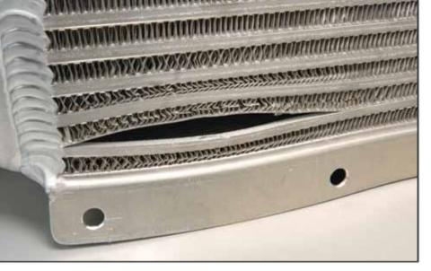
AERO-Classics pressure tests 100% of their coolers so customers won't experience this sort of failure. This opening was likely caused by surface contamination during cooler assembly, thus defeating the brazing process. All parts are vapor cleaned before assembly, but an occasional burst still occurs in testing.
