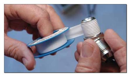
▲ AERO-Classics insists on steel oil line fittings, saying they never gall, unlike aluminum fittings that always do. AERO advises that Teflon tape is a good thread sealant, or Loctite Red can be used for more durable applications. Loctite will require heat to remove the fittings.
