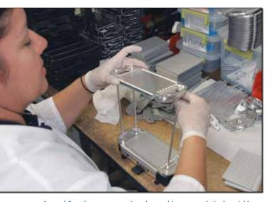
Assembling drawn-cup sections by stacking goes relatively quickly, as this AERO-Classics technician demonstrates. It also hints at why aviation oil cooler depth and width are standardized, with greater cooling needs addressed by adding more plates.
