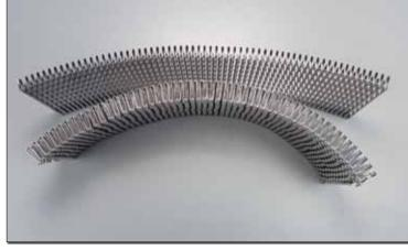
Comparing the drawn-cup air fins at top with the bar-and-plate fins at bottom shows the increased height and many more individual fins of the bar-and-plate design. Simply put, the bar-and-plate offers much more surface area to the cooling air.
