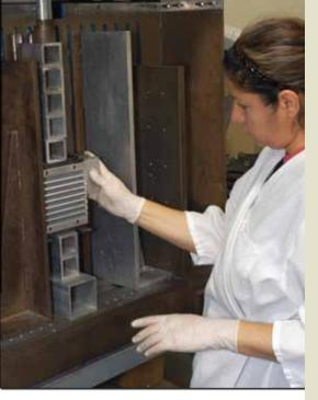
Bar-and-plate cooler cores are more tedious to assemble. The technician must hand-fit each plate, turbulator plate and bar, a stacking job done in this vertical press. Evening and squaring the assembly is done with small prying tools and gentle taps with an aluminum block. Ultimately the assembly is banded tightly together before going into the vacuum furnace.
