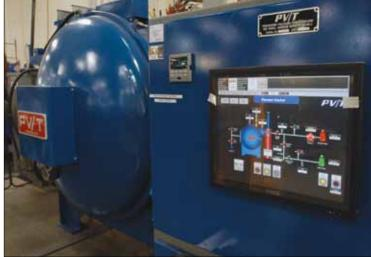
The round tank is AERO-Classics' vacuum-brazing furnace, where loads of coolers are heated to 1100° F in a near-perfect vacuum. This melts a micro-layer of brazing material previously deposited on the cooler parts, welding them into a single unit.
