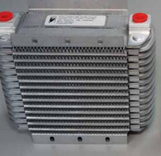
Nearly identically sized, AERO-Classics' Remote Mount (left) and High Efficiency (right) oil coolers are excellent representatives of drawn-cup and bar-and-plate cooler designs. Visual clues are the drawn-cup cooler has finned-end tanks and a more open air fin pattern, compared to the bar-and-plate cooler's smooth, hydroformed tanks and multiple welds.
