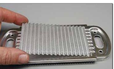
Simply stacking cups and turbulator plates is the basic building block of a drawn-cup-cooler. Typically seven or nine such rows are needed to cool a 150 to 200 horsepower Lycoming, but much depends on the installation and ambient temperatures where the airplane flies.
