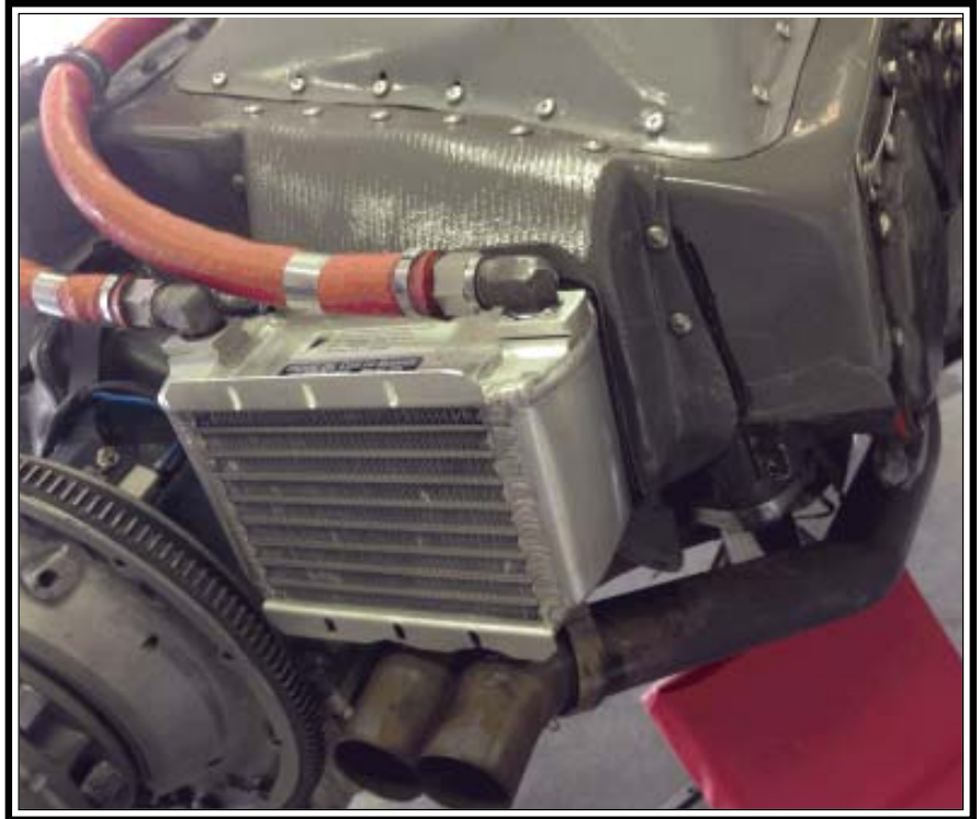
new smaller cooler fed from high pressure cooling plenum
