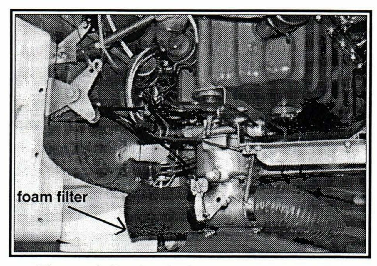
The new air filter location increases ram air capability and decreases the standard Aeroduct's drag. It may even allow more cooling air to the hotter running cylinders.
