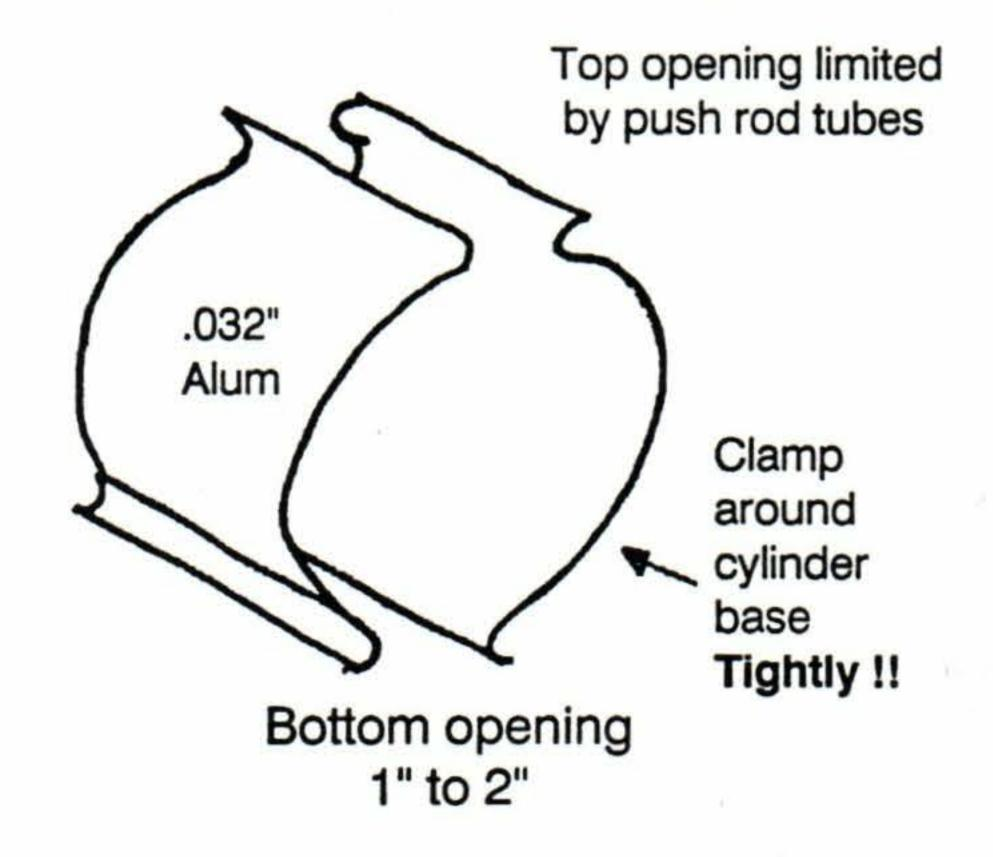
After each successive clamping, push the aluminum down 1/16" more and bend 30 to 50 degrees.
