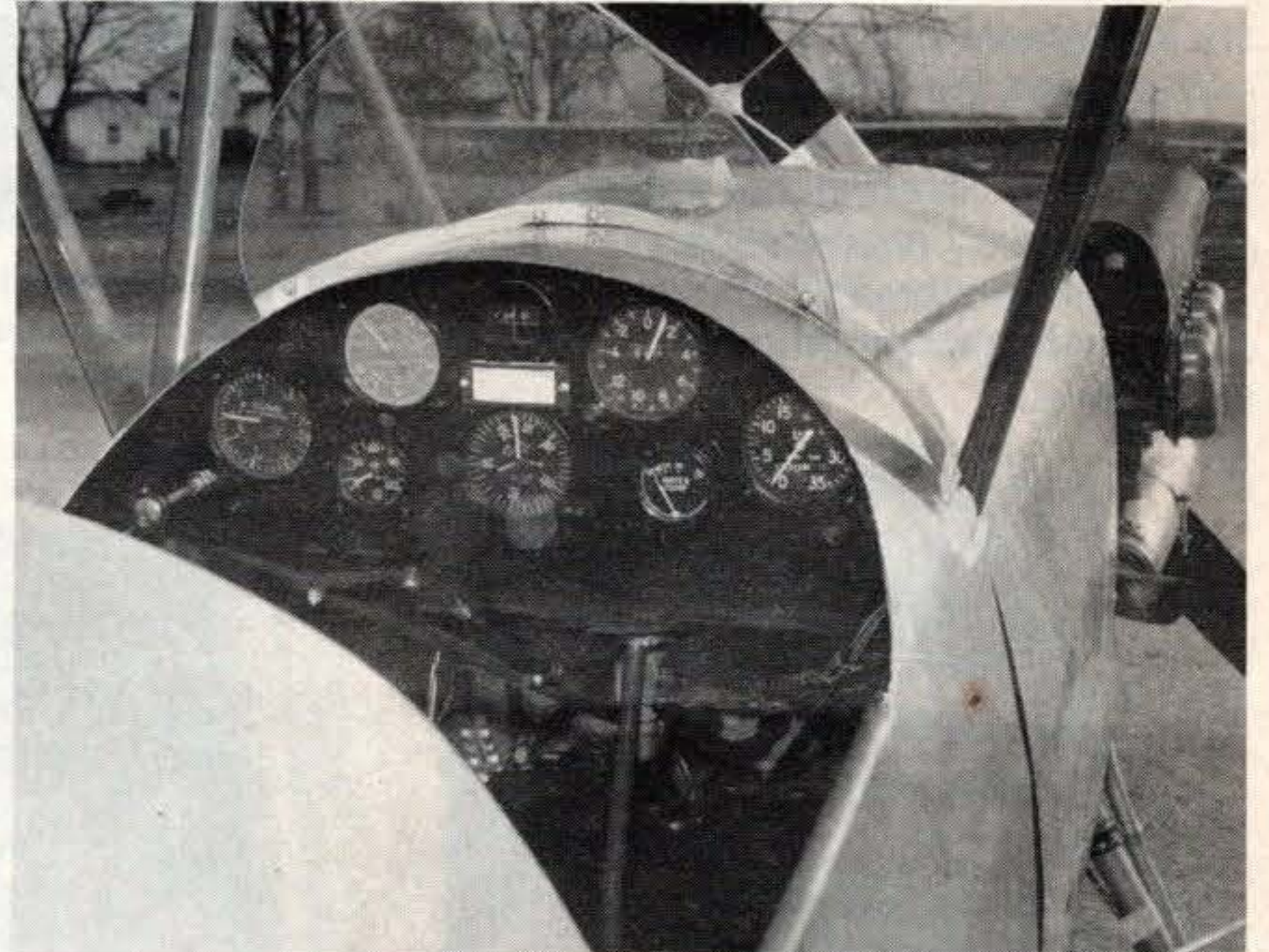
This simple panel also uses the "Indy car philosophy" with the stall speed indicator straight up. See center dial.
