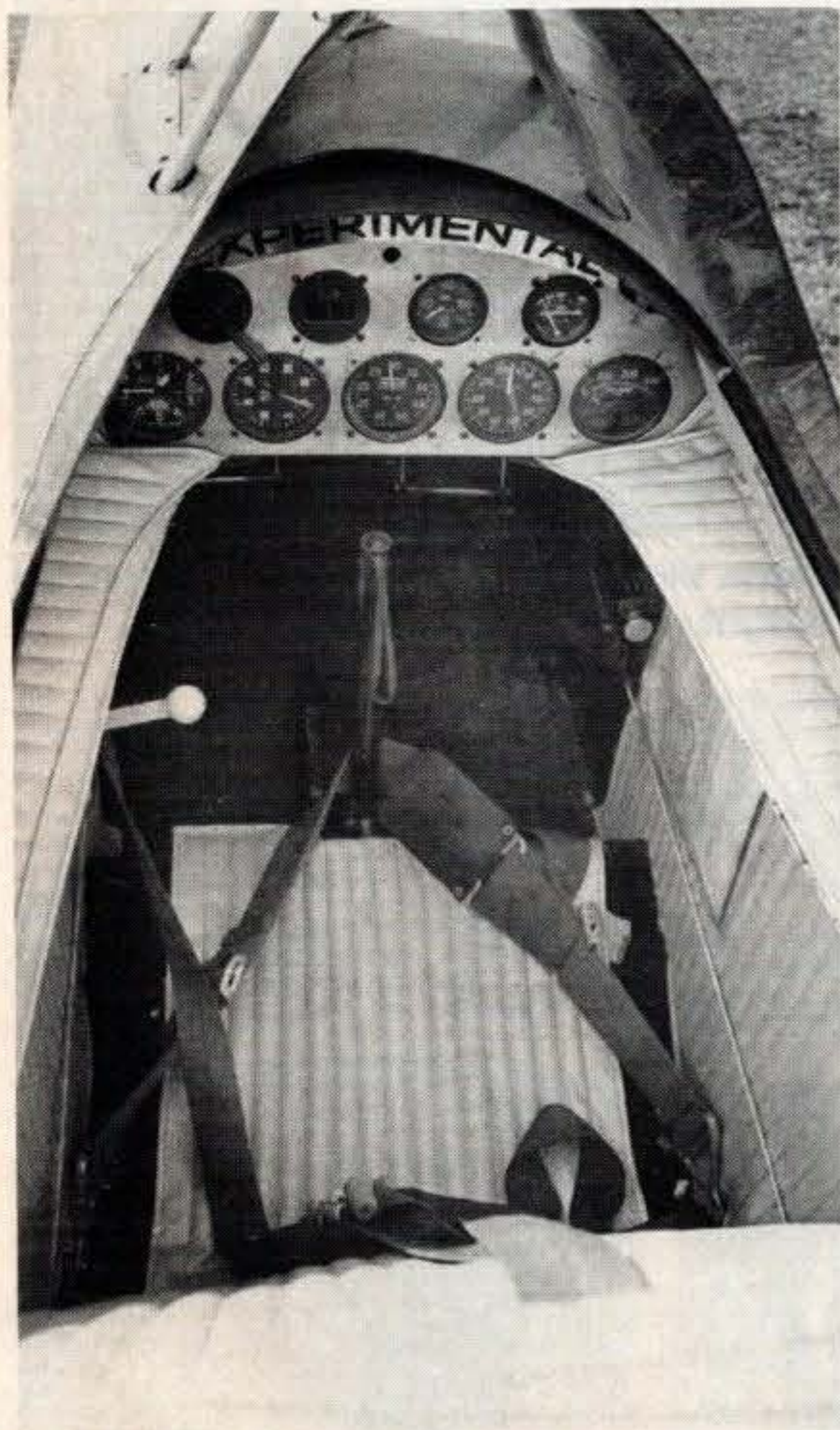
This light colored panel is free of switches and protrusions. The RPM gauge is like an "Indy" car . . . the needle is designed to be straight up when proper RPM is easily seen.
