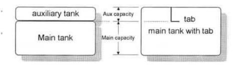
Refer to the column in the chart below corresponding to your fuel tank configuration. Tap the LF button to select one of the four following fueling choices on the left column of the chart.
