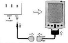
the small round plug of the JPI cable into the data connector on your aircraft instrument panel, and the cradle or travel cable to the Palm handheld.
