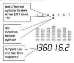
Continue leaning smoothly without stopping. With a vernier mixture control, turn the knob about a quarter turn every second. With a non-vernier or quadrant mixture control, lean slowly and smoothly about 1/16 inch every five seconds. Eventually, one cylinder will reach peak before any of the other cylinders. The EDM-900 will determine this automatically. Notice that this cylinder is not necessarily the hottest.
