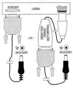
to a PC using a Palm<sup>™</sup> handheld as a intermediate courier, or directly to a laptop PC.
