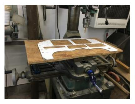
here you can see where I drilled the round holes with a lot of small holes to allow me to use the jig saw to open the circle up. Then using a air grinder with a rotary bit allowed for a reasonable accurate circle, then a 1/2 round final was used. A perfect hole for sure and overall, it took very little time to do. A sharp file cuts this grade of aluminum very quickly.
