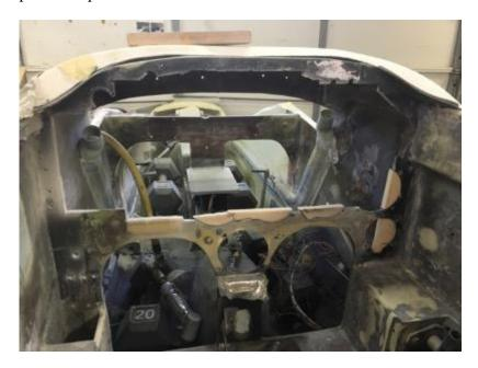
I like using .090" 67061-T6 aluminum. It is easy to machine, stiff enough for the purpose and most importantly, most set backs (exposure ring) of the instruments is designed for a panel of this thickness. You'll also need a basic computer drafting program (I use Auto-cad) which helps with the design of the panel and some basic hand tools such as a jig saw, drill, rotary grinder and band saw. That it!
