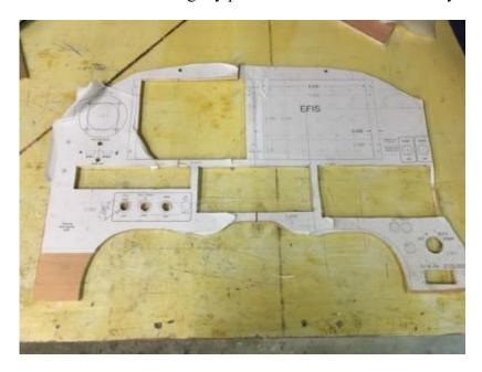
This is the panel pasted together with individual pieces of paper. No strength, just hacked and cobbled together.
