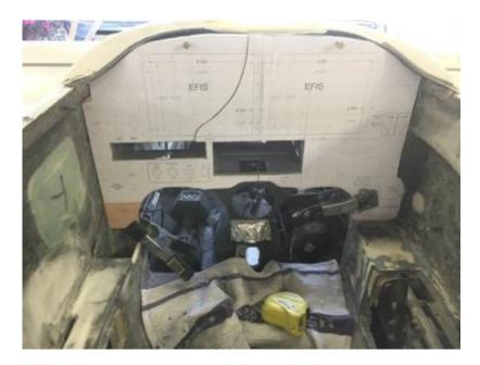
Here you can see I am not even worrying about the perimeter or strength. Just plunge cutting with the band saw to open the holes up. You end up with a panel that has no real structural strength, but will allow you check the fit and feel with the cans lightly placed. LOTS of issues with my first draft.
