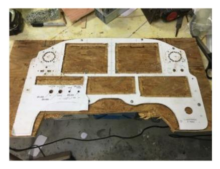
The panel is cut and ready to mount the radio cans. The cans presented a special problem due to the narrowness of the opening between the radios (3/8). My first attempt to mount the cans turned out to be total crap as all the cans were not level nor straight and wiggled around a bit.
