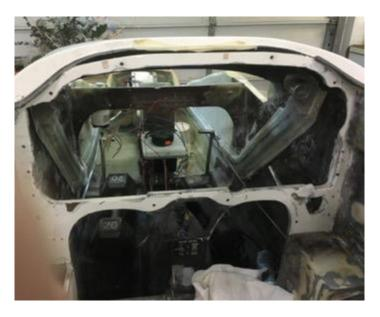
NOW you are now ready to cut the panel out. I think you can do it a number of ways. CNC, using a mill, or a jig saw (my choice). For this panel I used the jig saw first, then cleaned up the lines with a mill. Mostly the mill work was a waste of time.
