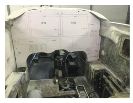
Hum, will the cans fit and was sort to problems to I have going on behind the panel? Yep, I had a number of unseen issues. With a bandsaw you can easily cut the working panel out in a minute or two since you aren't worried about destroying your 'working' panel.
