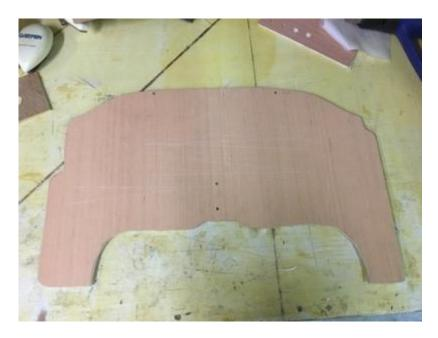
Next step is now that you have the basic panel made, you need to index it to the plane. On this picture you can see two holes at the top and middle of the panel. This panel becomes your your "Master Template". Transfer drill the alignment holes to the mounting flange. DO not drill permitter mounting holes at this time.
