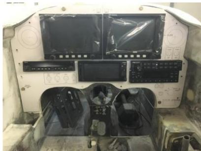
Now you have a good idea of interferences and problem areas. I needed to make all sorts of adjustments... such as switch location and vent locations (too high)...first iteration done. Back to the computer for to modify the drawing.
