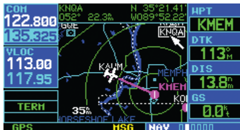
Figure 4-11 Panning Pointer Placed on Waypoint
