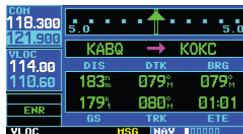
Figure 9-10 VLOC Coupled to External CDI
