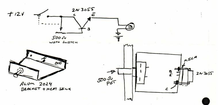
Use a mounting kit for transistor with mica washer and heat sink compound. Your bracket is the heat sink.
