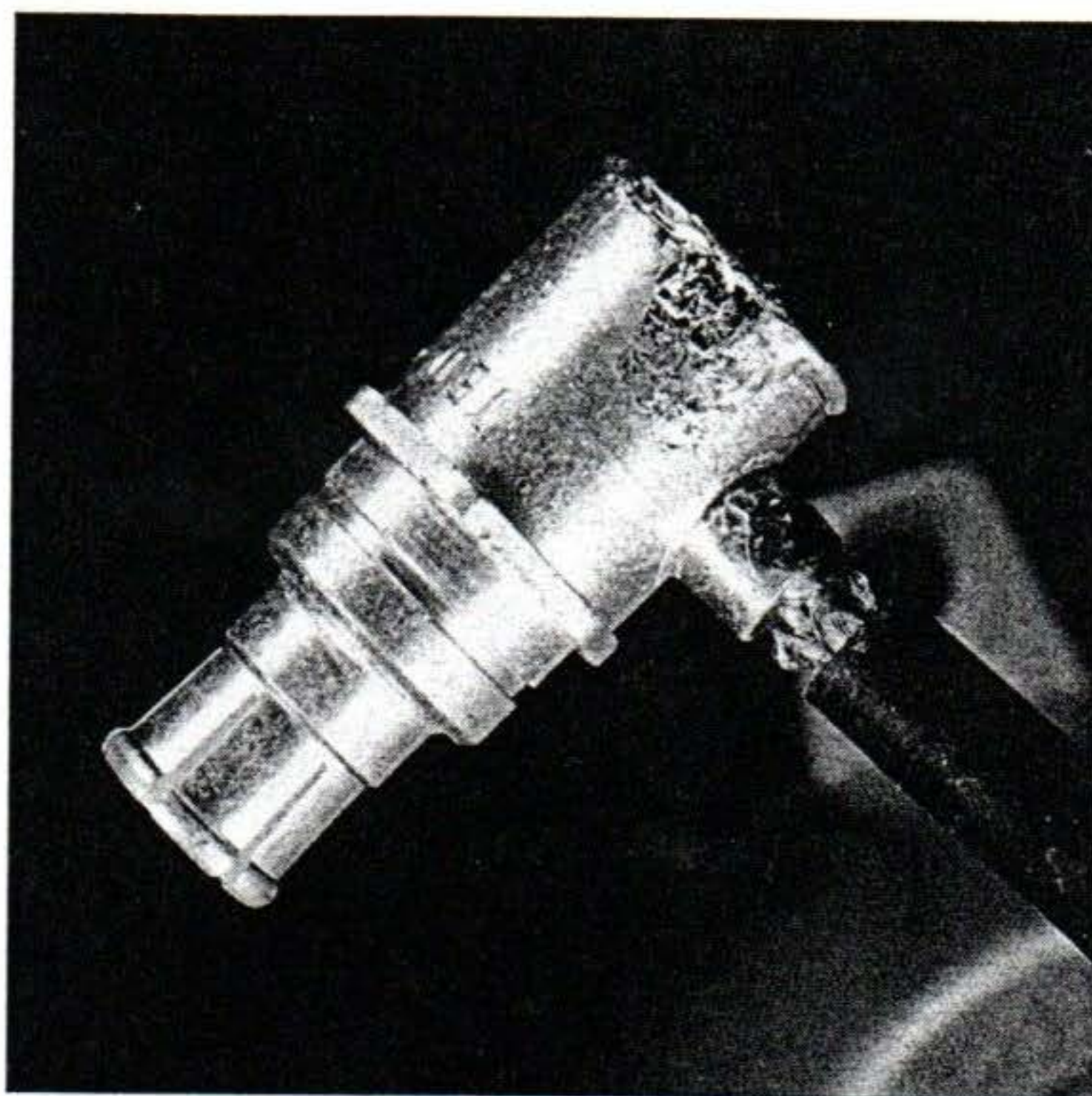
Photo 2. A coax elbow fitting eliminates the need to bend coax severely behind the panel.
