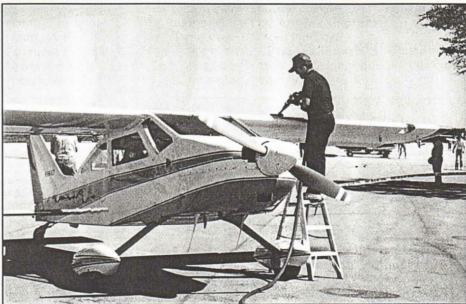
Fuel tanks filled to the top with cool fuel during low morning temperatures will overflow through the vents as the fuel and the temperatures warm up on a hot sunny ramp.
