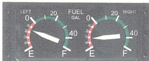
Defiant Fuel Indicator w/sump level
