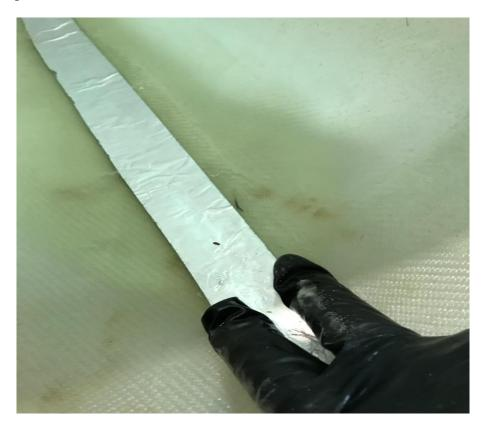
If you pull it back the aluminum strip on itself and use a wet brush to tamp anything that has come up back down the final picture looks pretty good - but you will need to sand edges. Again, if you have stretched the tape out with the aluminum off in this process - making it narrower, you can pull the threads straight and adjust its width again.
