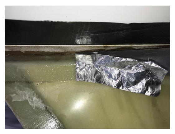
Then use the wet brush again to poke the BID tape against the surface, you really can't squeegee any epoxy out of these joints. You leave the cradle and pod in place to dry - you cannot use heat to cure the tapes - you can so easily melt the blue foam in the wing - not a good idea - particularly here.
