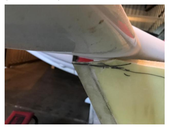
I used a stir stick to mark each side of the pylon…and eventually cut that back to a brush handle under the horizontal part of the wing and the stir stick on the curving leading edge. I followed this approach about 12 times. Eventually I got in the habit of making my marks and then sketched another  $\frac{1}{2}$ " of leading edge cut out. I used an angle grinder to carefully cut through the skin (biased upward in the foam and then used a flat sanding bar to bring the foam down to the level.
