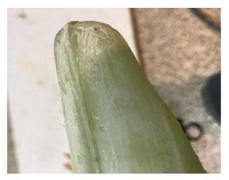
I thought I'd start with the leading bullet end of the pod and work along the bottom - nah - when I got to the pylon I realized it was well out of alignment. Getting the pylon parts to line up first resulted in the nose separating, not badly:
