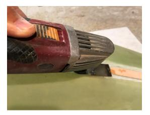
The front of one pylon was sketchy, so I sanded it back to run a new tape there - I added up the inches of un-covered baggage pods - and ended up with tin foil and about 45 inches of 3 ply of BID and a bit of 1 ply to cover the pylon leading edge I sanded previously.
