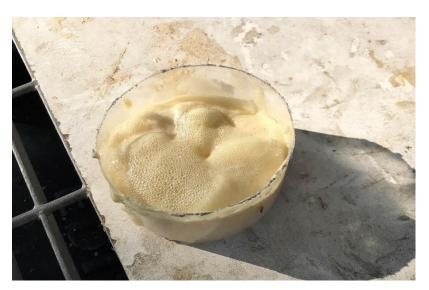
Well, the leading edge being so hard to fill, I put the nose down in the support box, installed the plywood strips and clamps - and mixed up a  $\frac{1}{2}$  cup x2 of the X-30.
