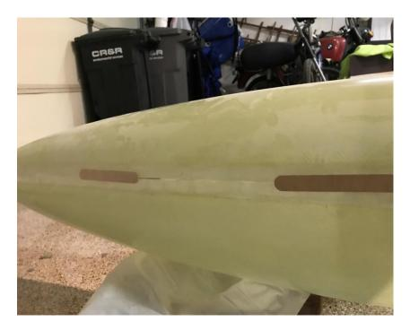
5. Assemble the tail cones first, and with the pods duct taped together, trail fit the tail cones to the pods.
