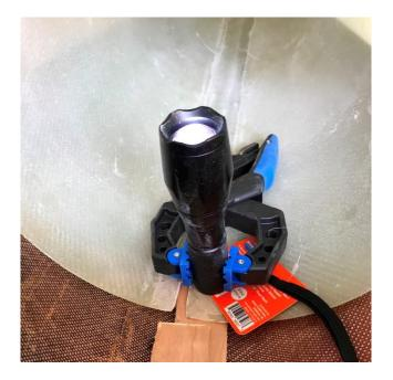
You can see the notch I made in the tail cone under the light. So using my Japanese draw saw along that part line allowed me to widen the cone to fit over the Pods.
