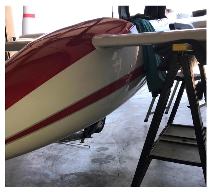
Then I tried cocking the nose wheel so I could run a chalk line from directly below the pitot to the prop centerline (in my case a little pointy spinner).
