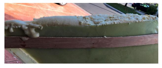
10. After the foam has hardened, remove the poster board from inside and top of the pylons, sand the foam flush with the inside of the pods, sand the glass dull around the foam,
