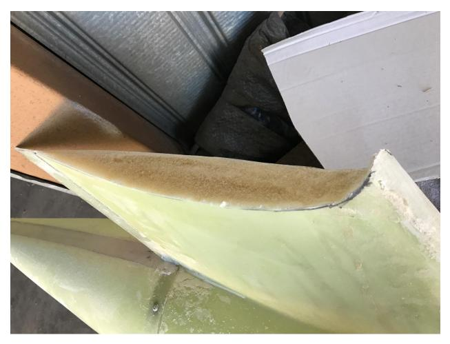
Obviously the cut out follows the right wing's sweep. Big step, sand the top 1" of the pylon before going on - and sand the soon to be exposed part of the strap too. In my case because I had to attach my strap by bolts, I removed them and replaced them as I sanded - and I put some clay (red) in the bolt to keep it clear of epoxy later with a brand new glassed strap that you apply, you don't have to do the bolts and anchors until after mounting the pylon to the strap:
