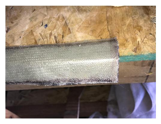
So with the tape up against both surfaces you use your gloved fingers to apply the tape firmly by pushing through the tin foil. When the tin covered BID tape is very much in place, you peel the tin foil back on itself - so it doesn't "suck" the BID tape of the surfaces and flox corner.
