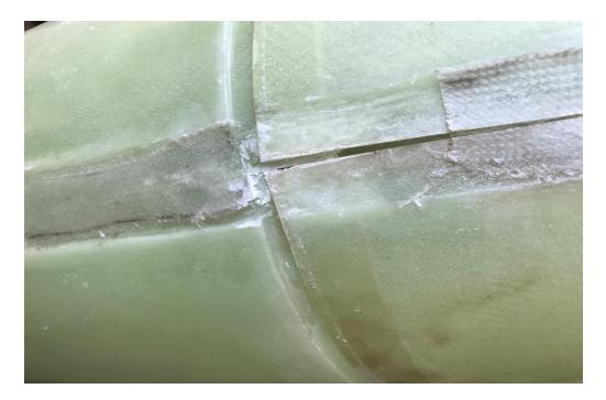
So you need to add some Bid to freeze it as expanded - yes you are making the cone slightly concave on the bottom as you do this. When you have let that Bid cure you can take the pod off and lay up Bid aft of the area where the pod is overlapped - you don't want to reduce the inside edge of the tail cone.
