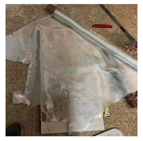
You can see the black lines on the tin foil under the glass. I cut the first layer out of the entire cloth, and then used the triangular remnants for the second layer (which goes against the parts) - the first layer on the tin foil is the final, visual, tape layer and looks a lot better uninterrupted, you can waste a lot of glass making the second layer one piece, so that's where you put the remnants. Here's the second layer:
