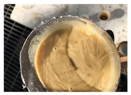
If you wait until the stuff starts expanding - you may run out of time, in my case I poured the first load in a long thin line from the leading edge to the trailing edge of the bottom of the pylon - ah, but it is hard to get into the leading corner. This is 5 minutes later - looking down in the pylon:
