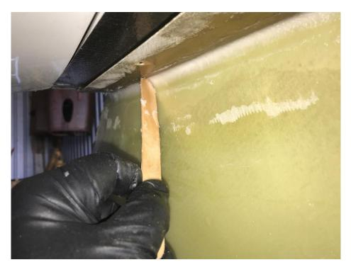
Again, you need to cut the tapes on the 45 - it will not go around tight spaces if cut at 90 degrees and will not be as strong as all the fibers going around the corner from the vertical pylon to the horizontal of the tape above.
