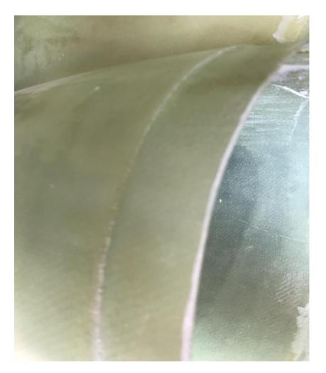
The other cone slid up to about 3/16'' from the available overlap. But the tight one only made it about ½ of the way on and I had to expand the built cone - I picked the bottom seam of the cone and installed a bright light in the tail cone so I could separate the parts on the seam:
