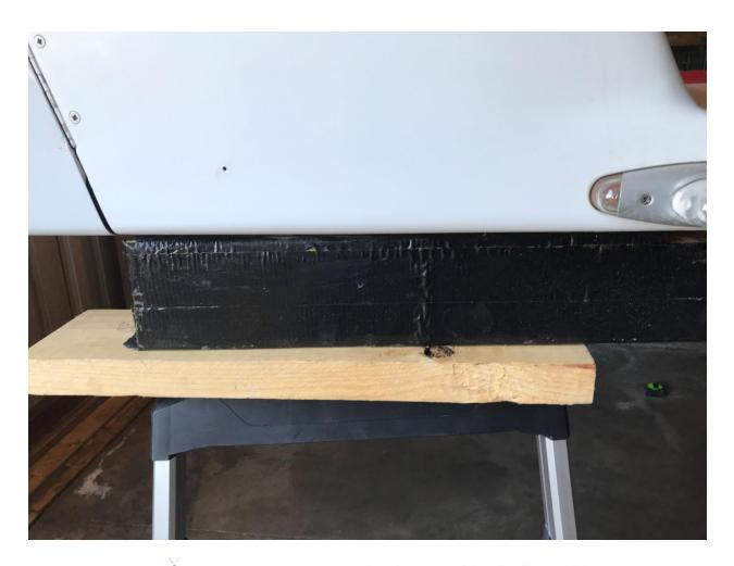
10. Using a Sears degree finder attached to a fuselage longeron, determine how many degrees up the nose of your plane is in level flight. On the ground, raise the nose of the plane to match the flight degrees. Most are 1-1/2 degrees.
