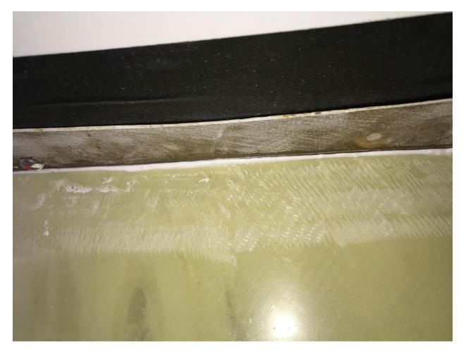
Then the flox corner using again, a single squirt of epoxy, but before you put cotton flocks in the mixture you use a brush to prewet the two surfaces you will be applying BID tapes to then you mix in the cotton flocks which mixture is then called flox. Here's the consistency I like:
