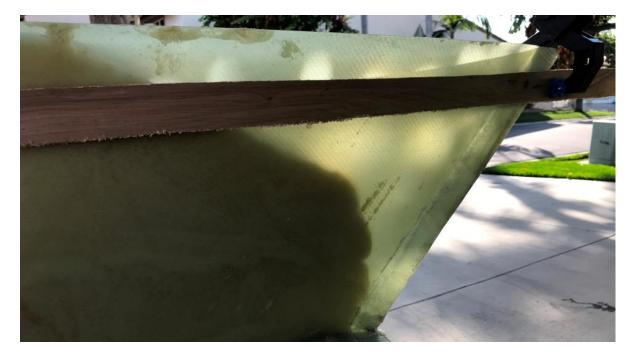
the first cup continued to expand, the second mixing cup was starting up and the first fill was pushing through the bottom tape a little:
