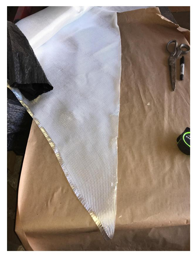
I build the BID tapes in advance, but it is not vital if you keep building - and here I also build them on marked Aluminum foil and then fold them about 90 degrees down the length of the tape so that it is ready to be applied.
