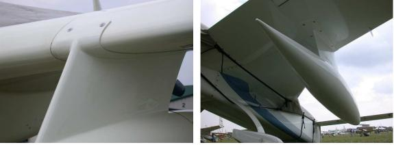
Although they have been primarily mated to the main wing of canard style aircraft, they can be mounted on conventional tractor aircraft as well – either under the wings or as a single pod on the bottom of the fuselage. Load bearing hard points may be required.
