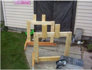
As you can probably see, each of these jigs has large carriage bolts through the feet. These can be adjusted to raise or lower the forward and aft parts of the jig to adjust angle and height. Caution—this approach will add time to your operation—lots of time, but it was fun to work with, and actually did a good job for me. The jigs were stable, and I also bondoed the "feet" to the cement to keep anything from moving. I think the jury is still out on whether or not I have OCD: ).
