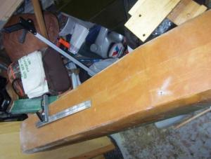
Then, the alignment. I wanted to do the whole expanse in one shot—not just one wing and then the other. I used 6 jigs to do this—2 each copies of the lower half of wing jigs #2 and #4, and 2 to hold the spar. (see below).
