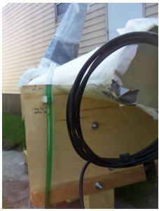
I had glassed my wing level boards on all 6 sides to discourage warpage, then used dabs of dry micro on the wing as bases to glass these level boards to the wings for a stronger and more stable hold. I knew it would be a long time between finishing the wings and doing the match drill, so I wanted to prevent issues.
