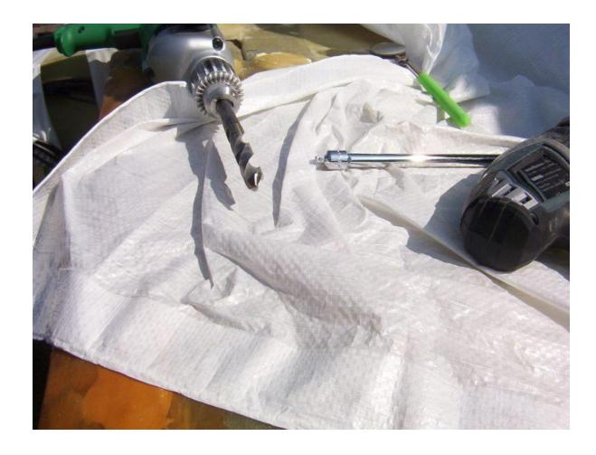
I then used the 5/8" reamer to complete the process, while the spar box was still in contact with the wings. Having done that, I both cut and pried the glass away from the micro dabs on the wings and spar, separated them, and whisked the micro from all parts.
